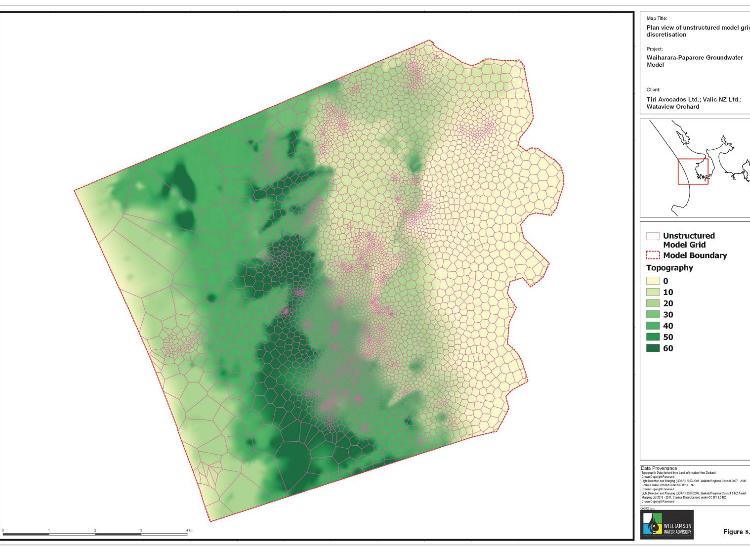
Plan view of unstructured model grid discretisation
