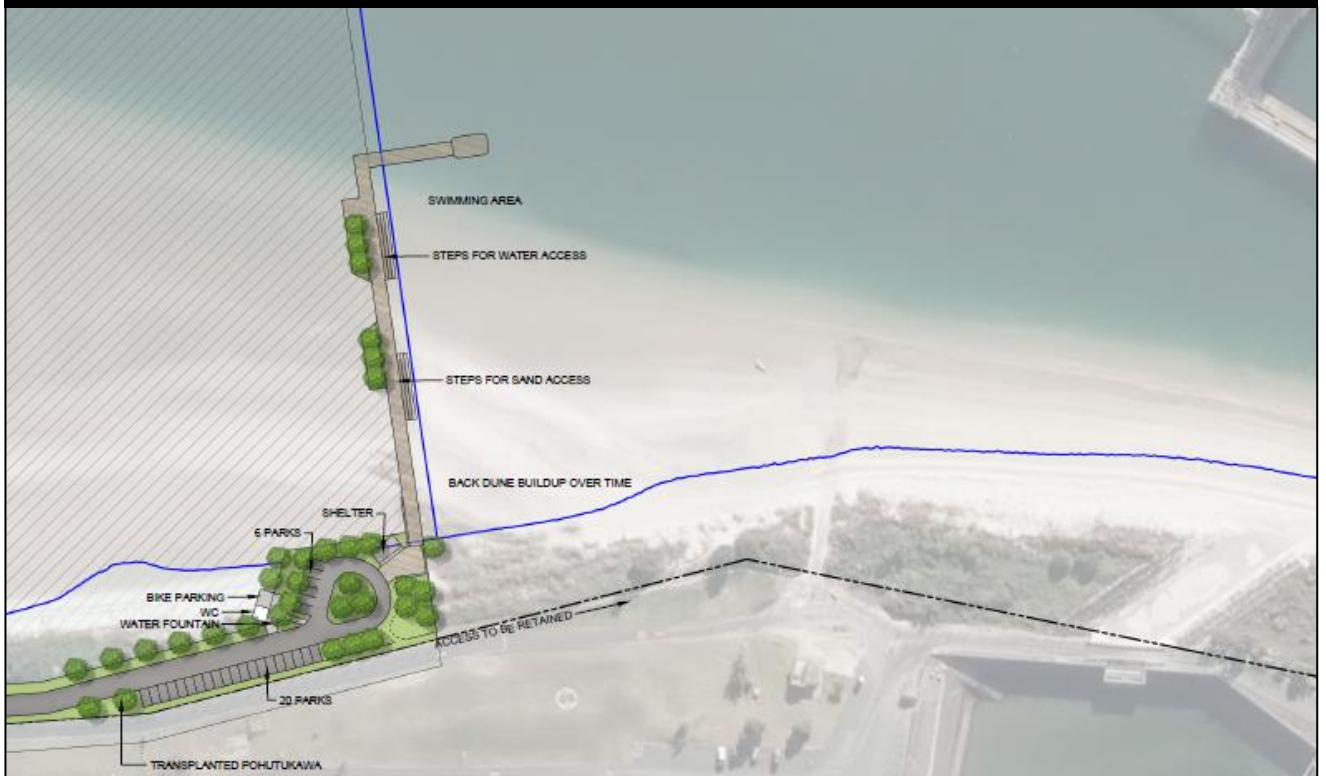
Figure 5: Proposed basic components of public access facilities at the eastern side of the reclamation
