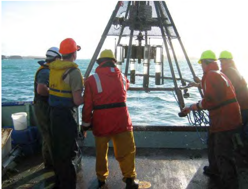
Figure 2-2: R.V. Kaharoa, Bay of Islands, August 2009. Retrieving the Multicorer tripod used to collect short cores at deep-water sites (photo: Lisa Northcote, NIWA Greta Point).
