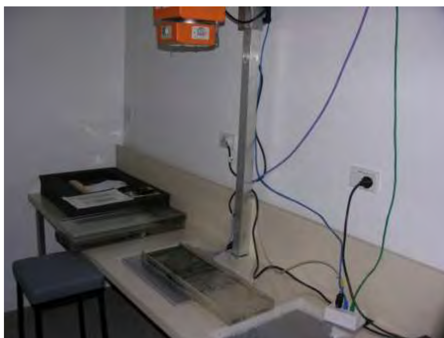
Figure 2-5: NIWA digital x-ray system, with a sediment slab mounted on the detector plate ready for imaging. (Photo: Ron Ovenden, NIWA Hamilton).
