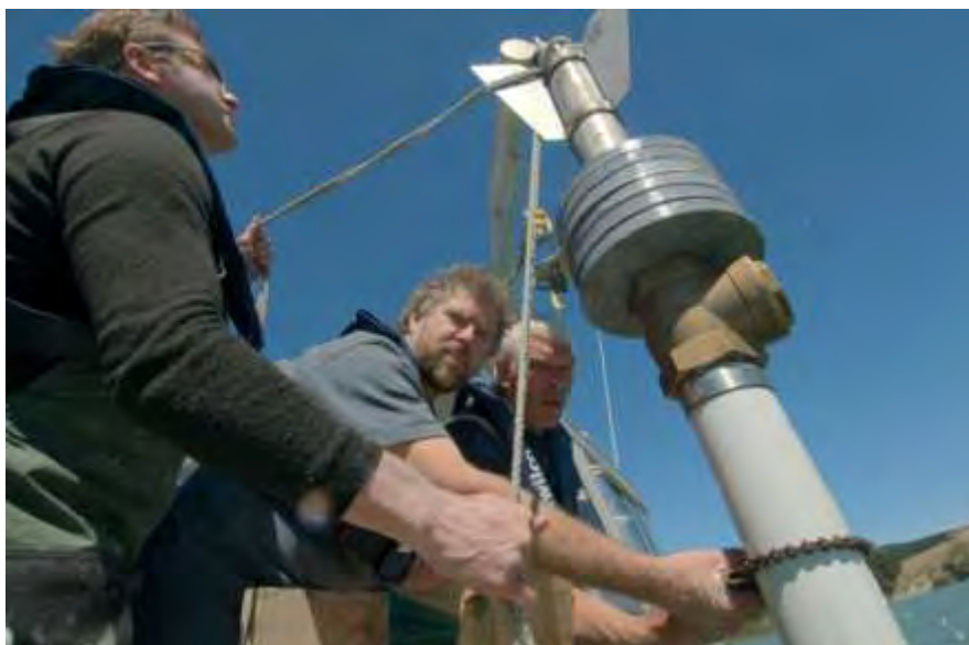
Figure 2-3: R.V. Rangitahi III, Bay of Islands, September 2009. Retrieving the Gravity Corer used to collect long cores at shallow-water sites (photo: Rod Budd, NIWA, Hamilton).
