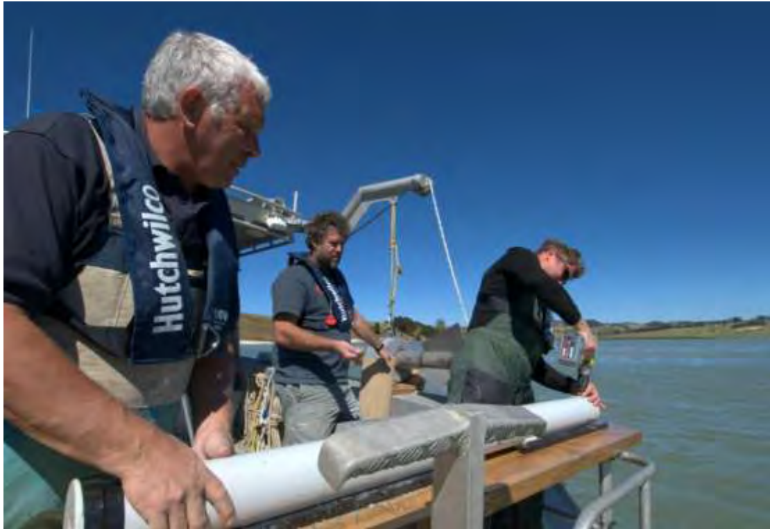
Figure 2-4: R.V. Rangitahi III, Bay of Islands, September 2009. Sealing a sediment core ready for shipment to NIWA Hamilton (photo: Rod Budd, NIWA Hamilton).
