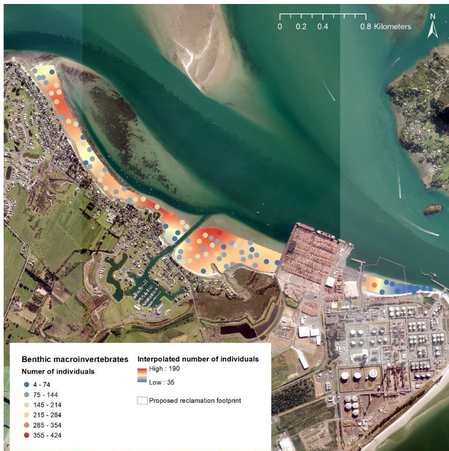
Figure 2: Example of a heat map showing total counts of all benthic macroinvertebrates obtained in core samples collected from Marsden Bay.
