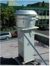
While  $PM_{10}$  levels at Robert Street are monitored using a Beta Attenuation Monitor (BAM), which continuously samples the air onto a specially prepared filter tape. The BAM is connected to a computer which records a result every 10 minutes. The data is periodically downloaded and converted to 24 hour averages (midnight – midnight).
