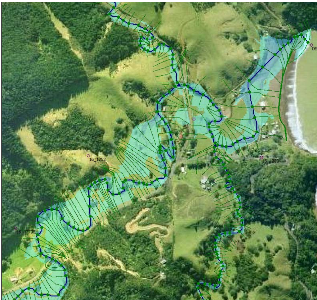
Figure 7-7 Example: Flood Compartment
