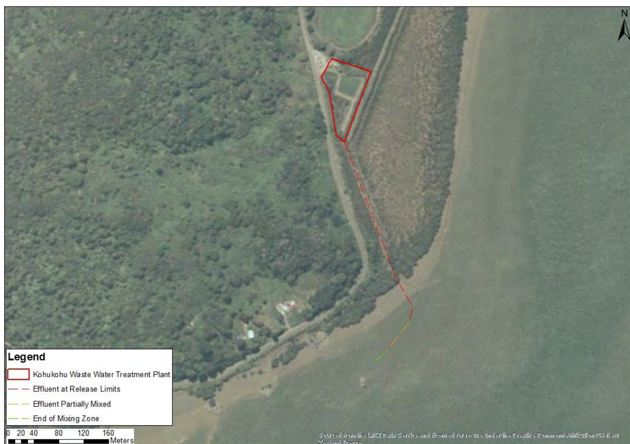
Figure 4: WWTP release points and mixing process
