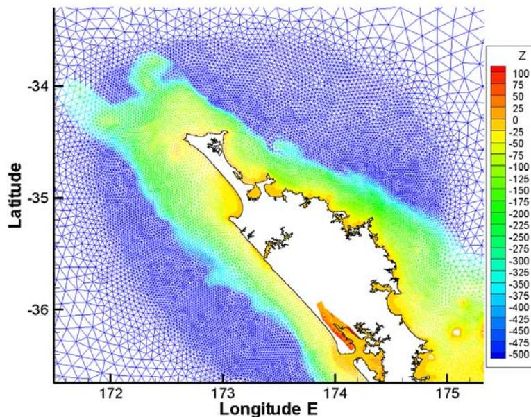
**Figure 3:** Close-up of the Region 2 grid around Northland. Colour represents water depth. The size of the elements can clearly be seen to grade in towards the complex coastline.
