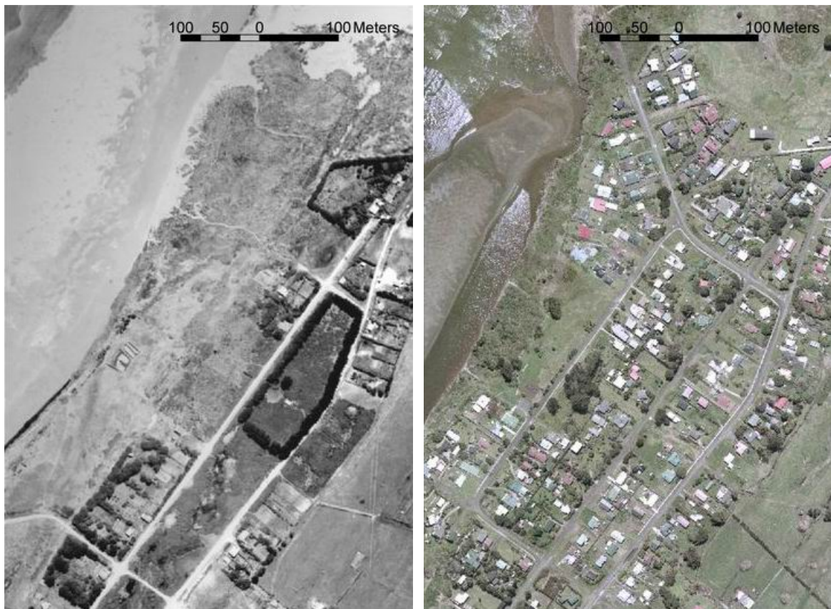
Development of the Ahipara foreshore from 1950 (left) to 2004 (right) with inadequate setback to allow for natural variability in the position of the shoreline.
