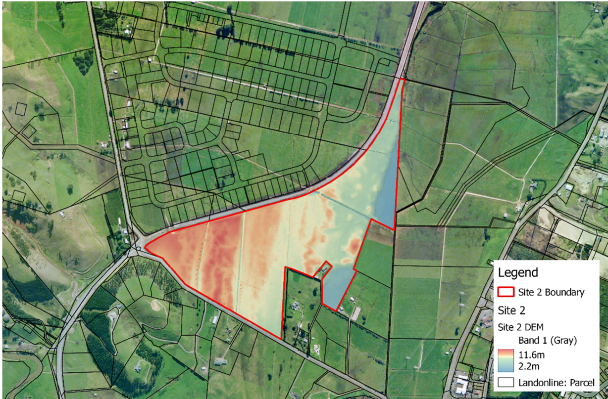
Figure 4. Site 2 Existing Terrain (Preliminary Civil Design)
