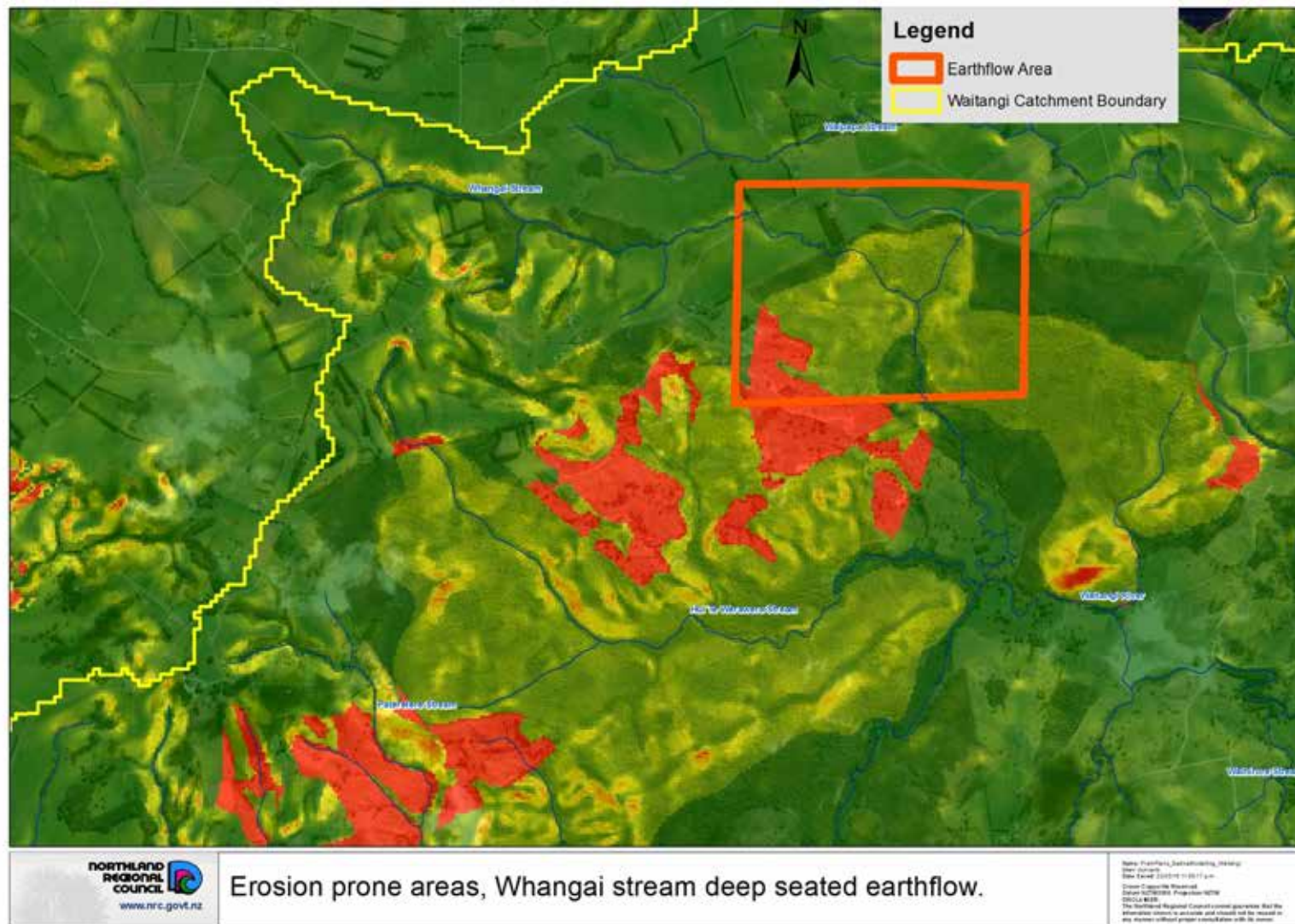
Figure 9: large earthflow on Whangai Stream.
