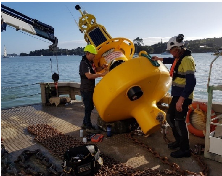
In 2020, NRC installed an offshore wind and wave data buoy outside the Bay of Islands harbour, to monitor conditions outside the harbour, to assist with the safe pilotage of cruise ships and to help commercial and recreational vessels heading offshore.
