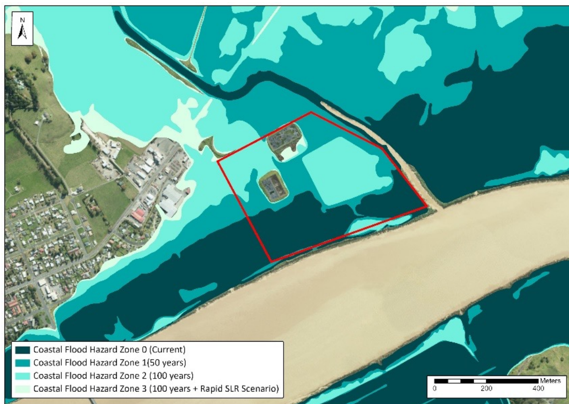
Dargaville wastewater treatment plant is located within both a river hazard zone and a coastal flood hazard zone.
