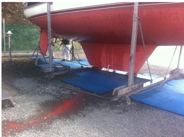
Elevated metal contamination is often associated with point source discharges at boat maintenance facilities.
