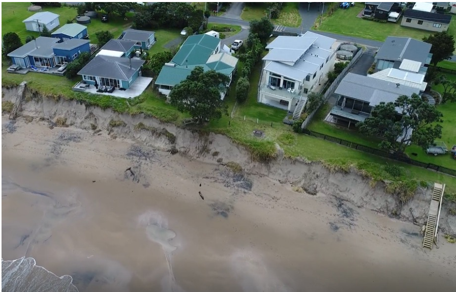
Residential development at Wellington's Bay (Whangau Bay) has occurred too close to the shoreline, leaving properties vulnerable to erosion during storms.
