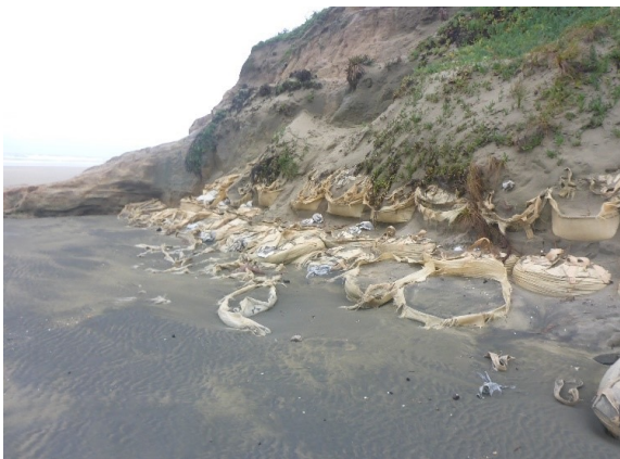
Left: The failure of sandbags installed in 2015 for erosion control, releasing thousands of broken pieces of polypropylene fibres along Bayliss Beach. Right: A pontoon that broke up during a storm released thousands of polystyrene pieces along the foreshore of the Cavelli Islands in 2014.
