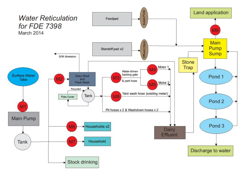
Figure 2: Schematic showing meter placement on Waiotu Farms Ltd.
