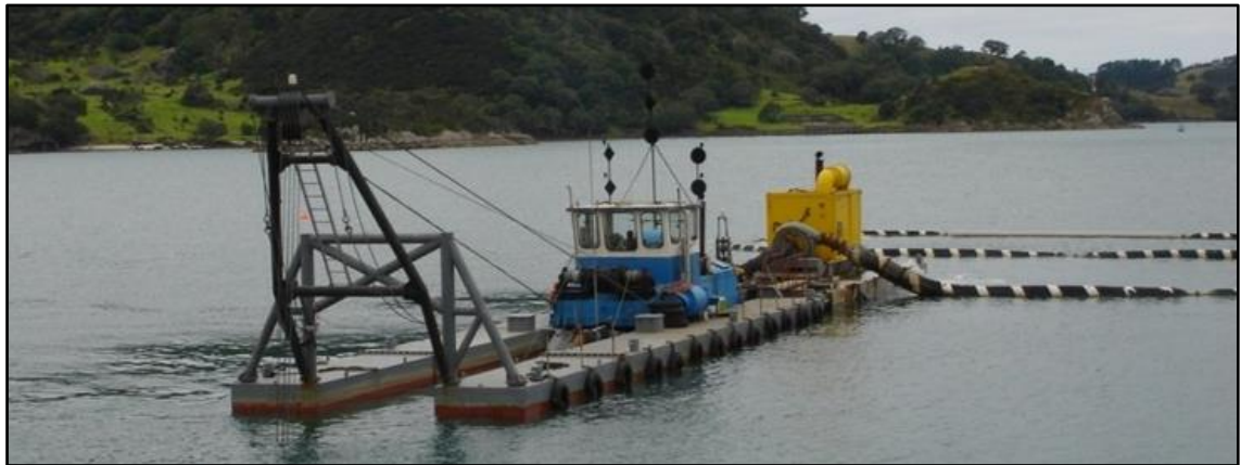
Figure 14: Small Cutter suction dredger with attached pipework
