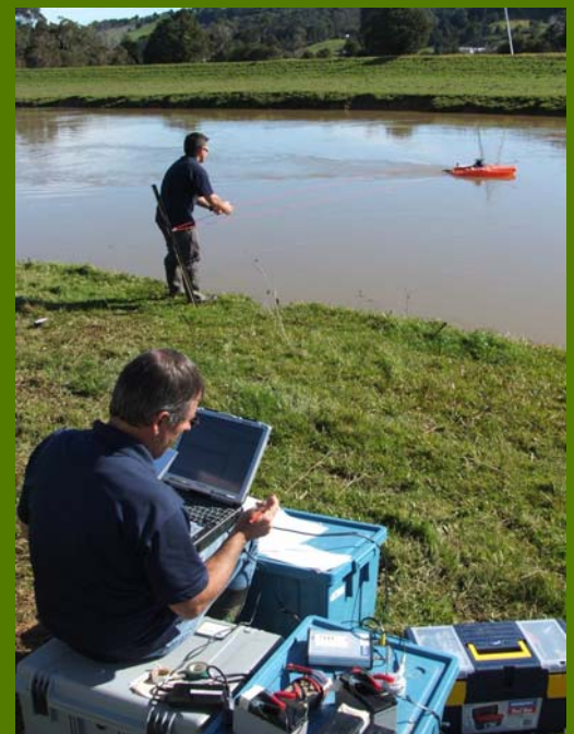
Northland Regional Council Monitoring staff measure high flows in the Whakapara River with an Acoustic Doppler Current Profiler (ADCP).
