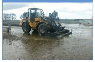
Washdown options include hoses or flooding systems. Figure 4.3-2 shows a flood system in operation. Flooding and hosing use comparable amounts of water, (flooding slightly less than hosing). The volume of water required will be reduced where solids are scraped off first (refer to Figure 4.3-3). A 3m wide scraper blade is quick and effective.
