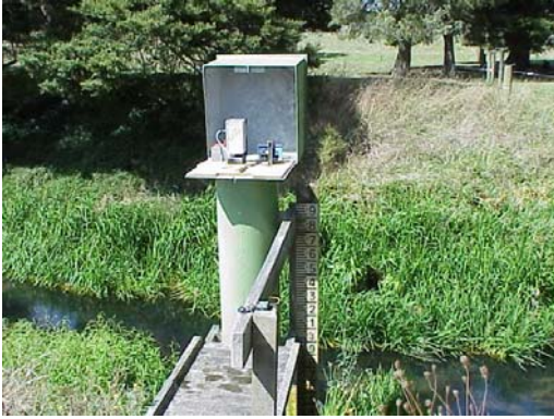
Water Level Recording Station – Waipao River at Draffin Road
