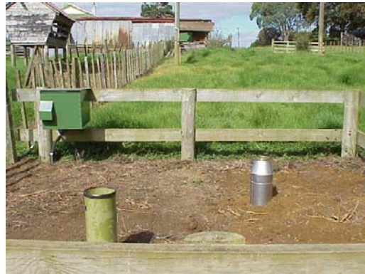
Automatic Telemetered Rainfall Station at Ohaeawai
