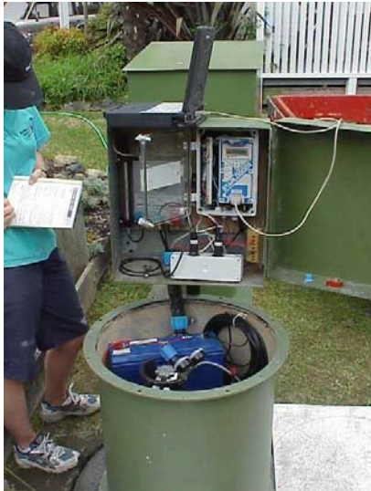
Russell Ground Water Monitoring Bore at Hananui Lodge. Recording Water Level and Conductivity
