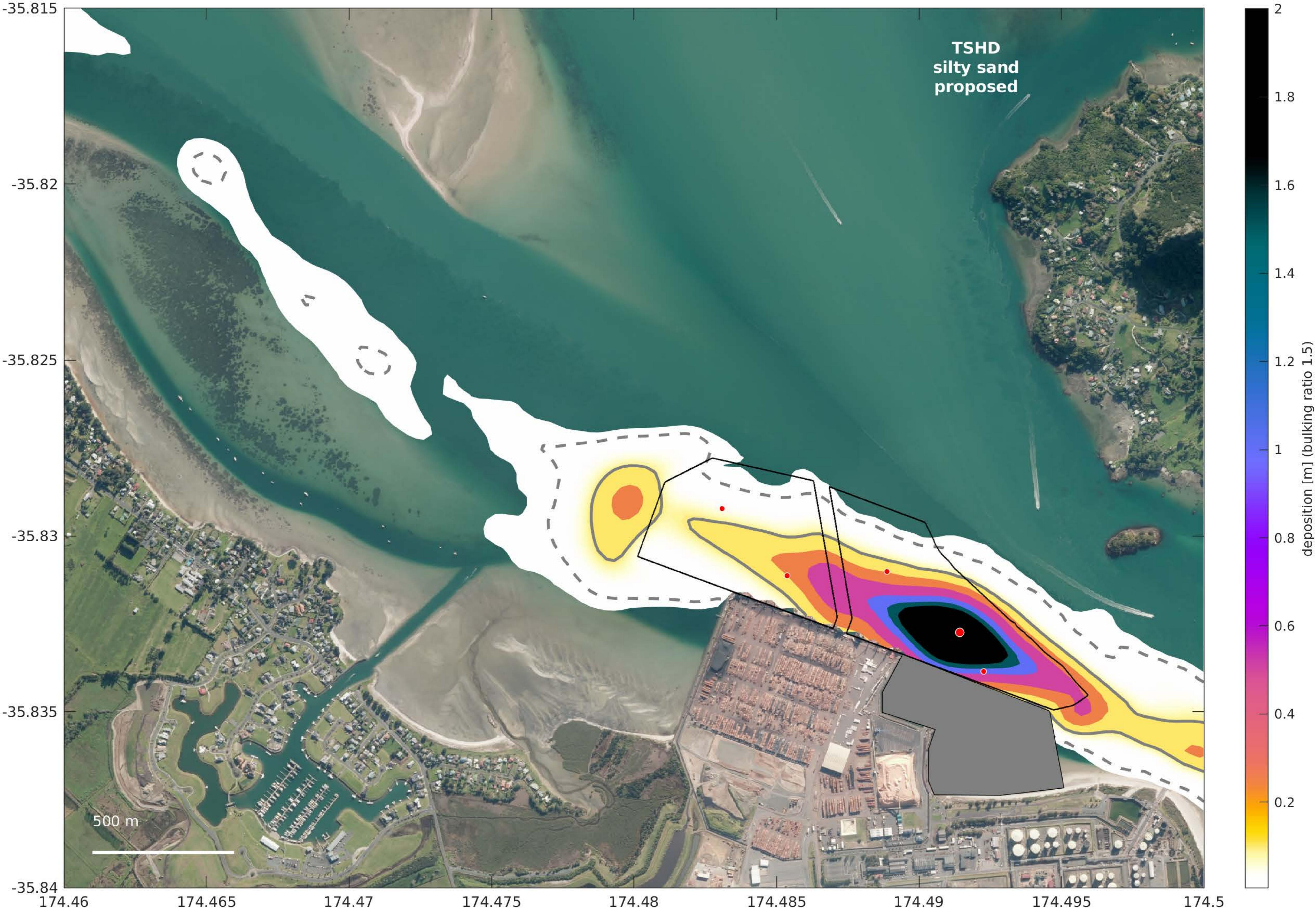
deposition [m] (bulking ratio 1.5)
