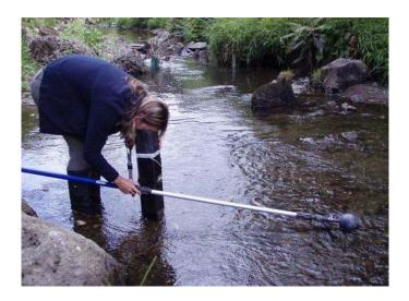
Photo: Council employee measuring water clarity downstream of a discharge
