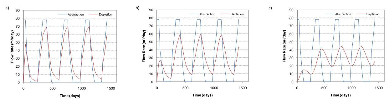
Figure 19. Abstraction and depletion rates for fractured basalt underlain by hard basalt with a) 35 m bore displacement, b) 200 m bore displacement and c) 1000 m bore displacement.
