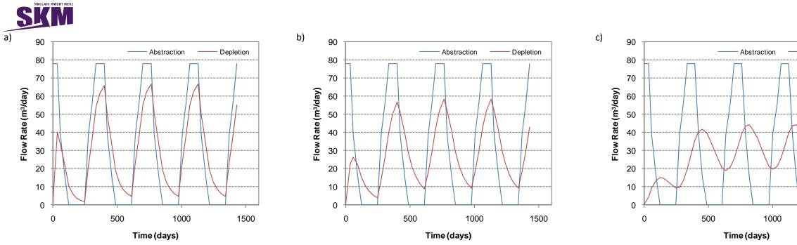
Figure 21. Abstraction and depletion rates for fractured basalt underlain by hard basalt with a fractured basalt zone with a) 35 m bore displacement, b) 200 m bore displacement and c) 1000 m bore displacement.
