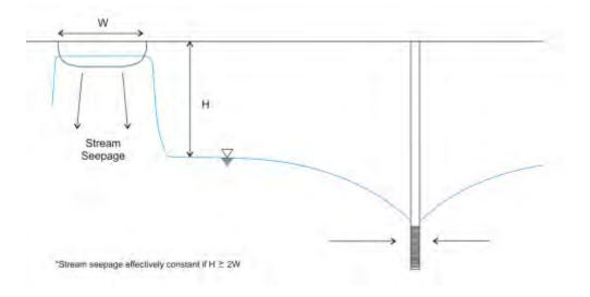
Figure 1. Bouwer stream seepage schematic.
