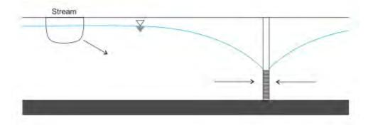
Figure 3. Hunt (1999) stream depletion schematic.
