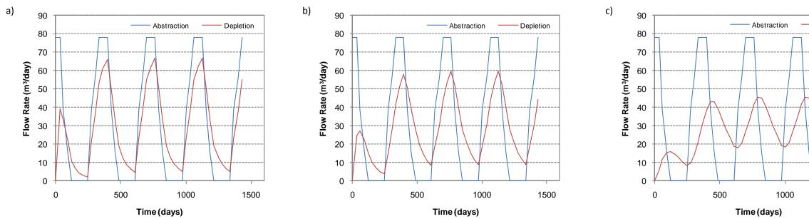
Figure 20. Abstraction and depletion rates for layers of fractured and hard basalt with a) 35 m bore displacement, b) 200 m bore displacement and c) 1000 m bore displacement. •
