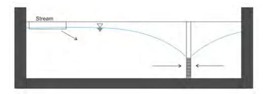
• Figure 4. Butler (1999) stream depletion schematic.
