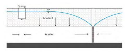
• Figure 11. Hunt and Smith (2008) spring depletion schematic.
