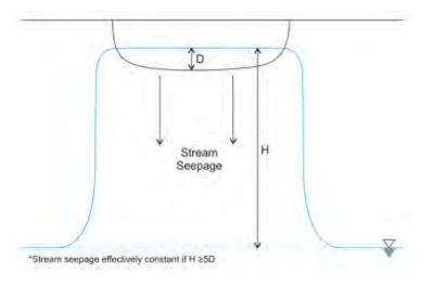
Figure 2. Hunt Flow Net Analysis schematic.
