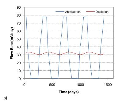
• Figure 22. Abstraction and depletion rates for hard basalt with a scoria zone with a 200 m bore displacement.
