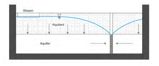
Figure 6. Hunt (2007) stream depletion schematic.
