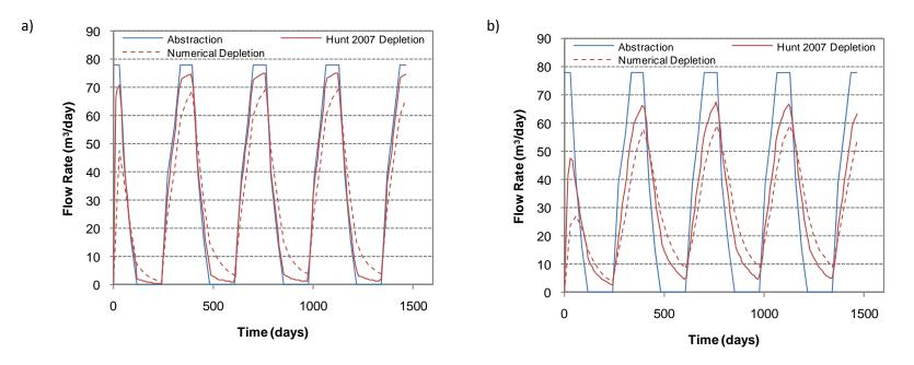
Figure 27. Stream depletion rates for numerical and Hunt (2007) analytical methods for fractured basalt underlain by hard basalt with: a) 35m bore displacement, and b) 200 m bore displacement, with a boundary at 800 m.
