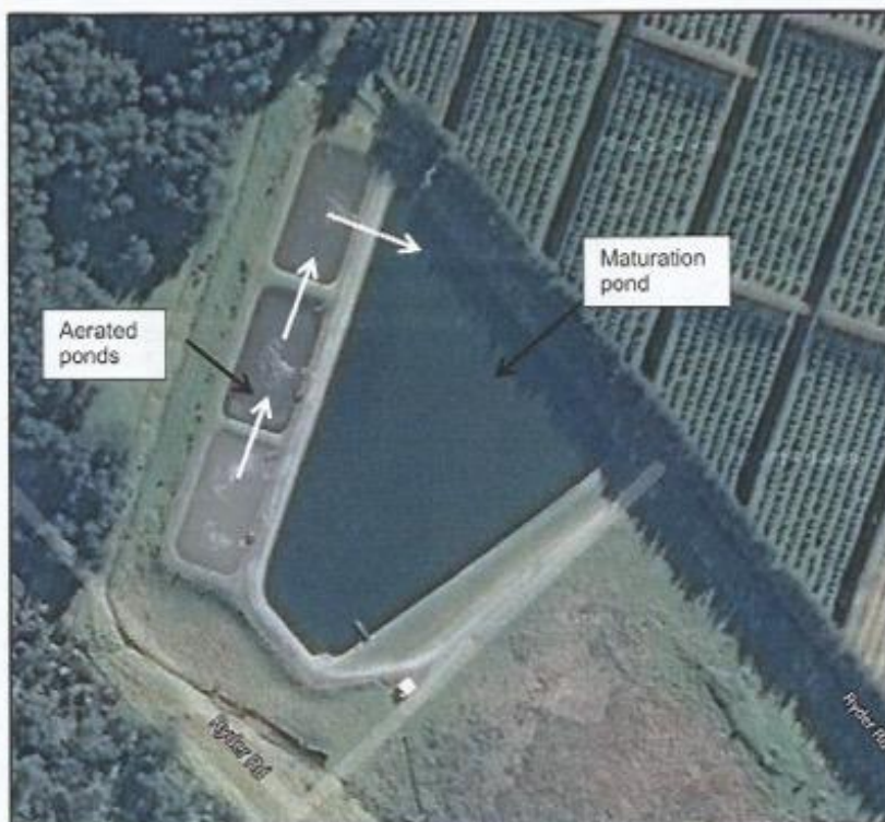
Figure 1. Aerial imaging showing the Taipa wastewater treatment plant. White arrows show the flow direction of wastewater.
