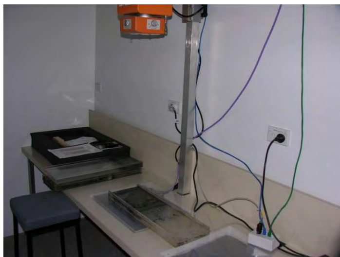
Figure 2-3: NIWA digital x-ray system, with a sediment slab mounted on the detector plate ready for imaging. (Photo: Ron Ovenden, NIWA Hamilton).
