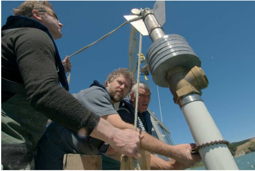
Figure 2-2: Sediment coring from R.V. Rangitahi III. Retrieving a Gravity Corer as used to collect sediment cores from Whangarei Harbour (photo: Rod Budd, NIWA, Hamilton).
