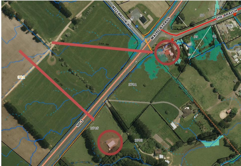
Figure 2: 250 metre setback from the boundary of a separate site that contains a sensitive activity (Residential)
