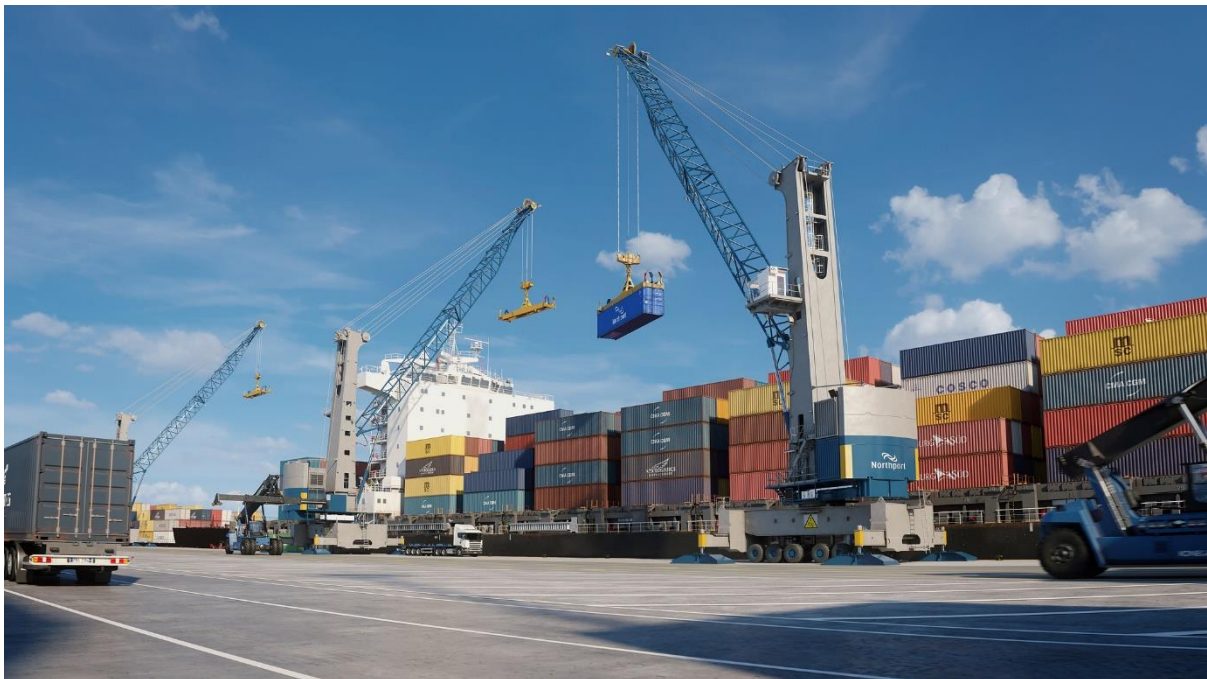
Figure 45: Simulated image of mobile harbour cranes (MHC) operating a vessel (Source: Build Media Ltd).
