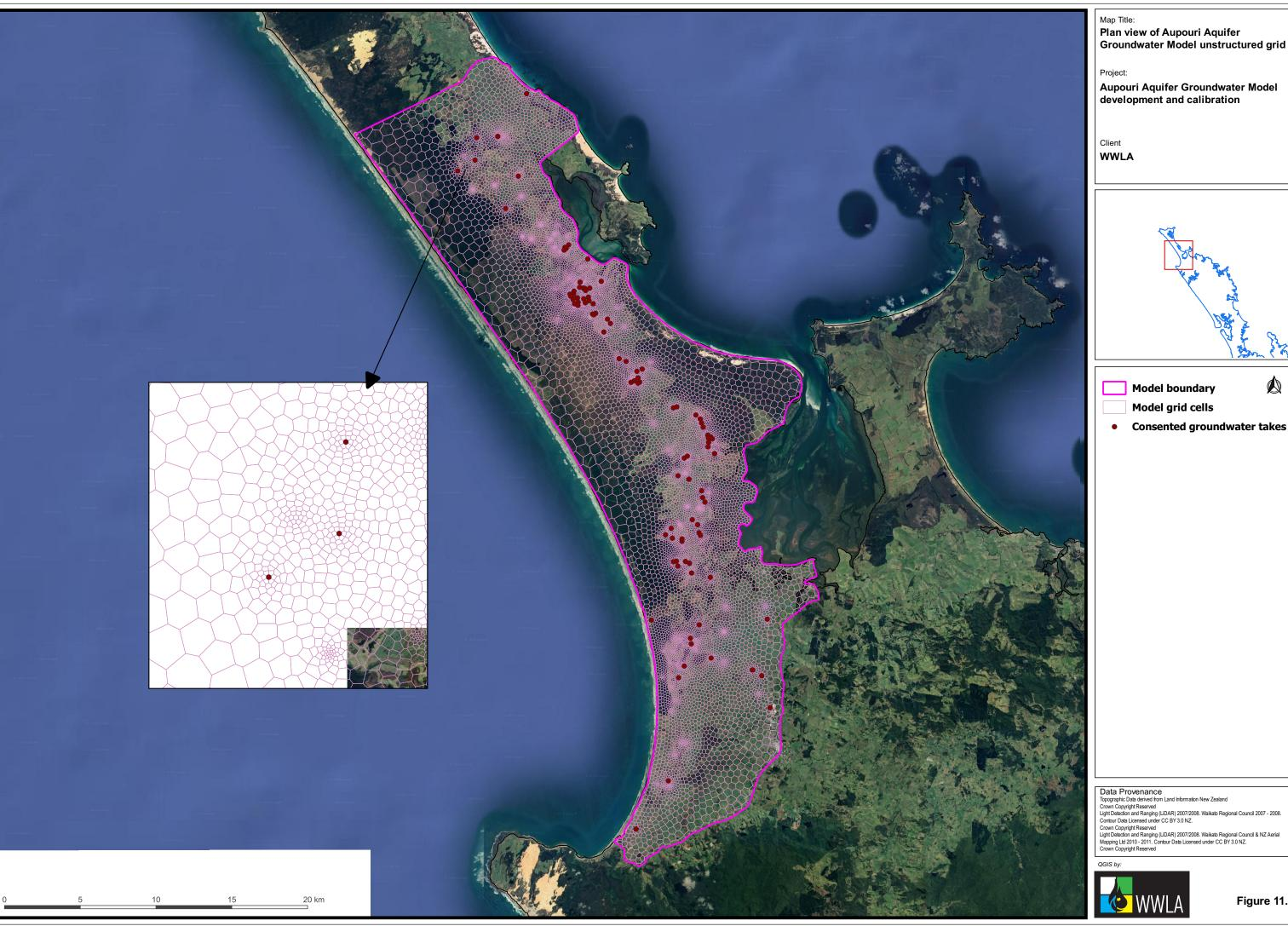
Plan view of Aupouri Aquifer Groundwater Model unstructured grid
