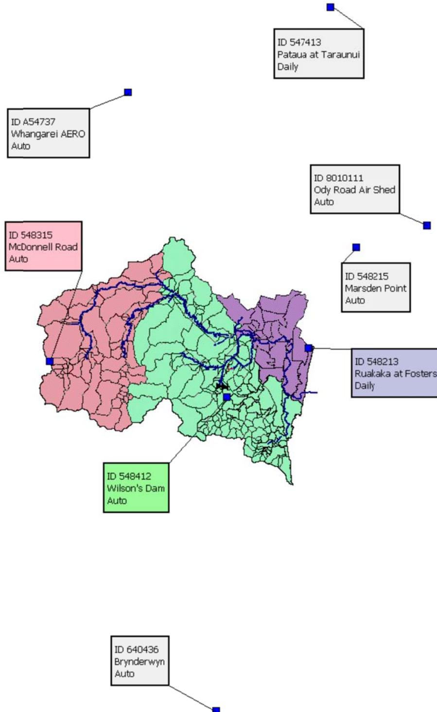
Rain gauges 548315 (auto), 548412 (auto) and 548213 (daily/estimated pattern) were used as inputs to the model for calibration. The following figures show the rainfall intensity and accumulated rainfall of these three rain gauges.
