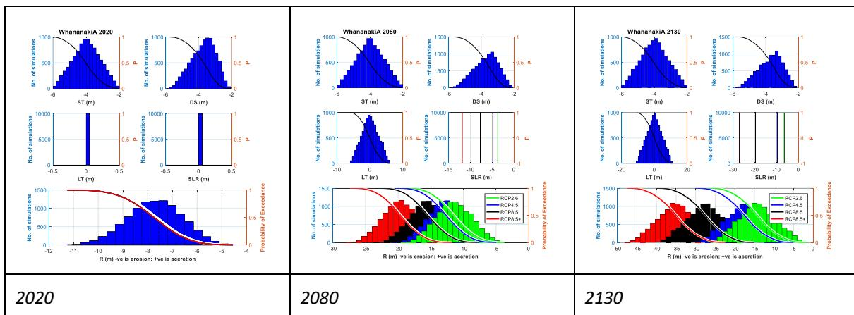
Figure 13-1 Histograms of parameter samples and the resultant shoreline distances for 2020, 2080 and 2130 timeframes for cell 13A
