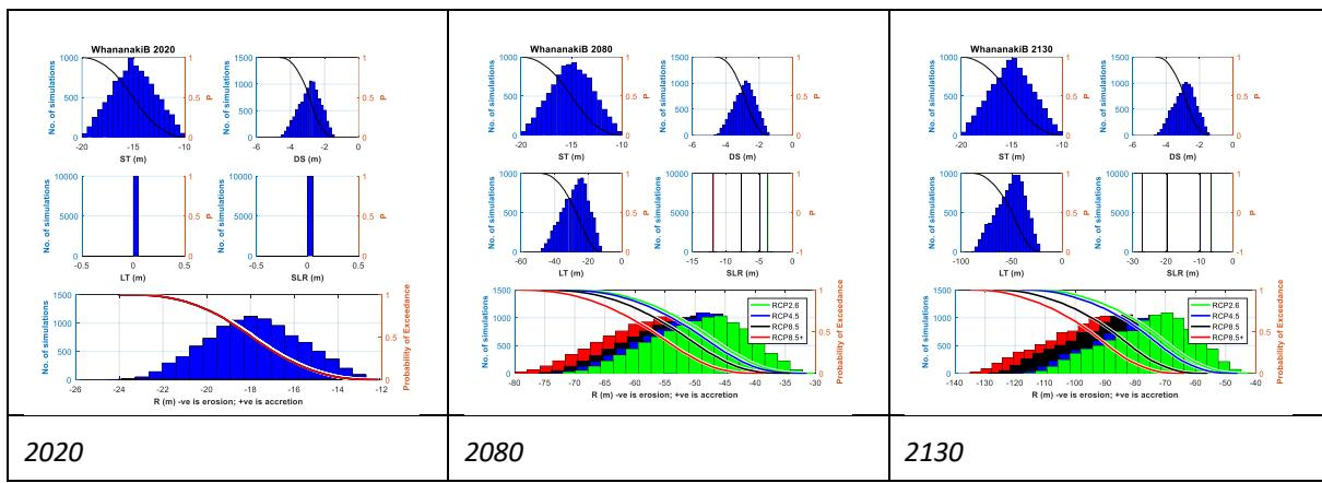
Figure 13-2 Histograms of parameter samples and the resultant shoreline distances for 2020, 2080 and 2130 timeframes for cell 13B
