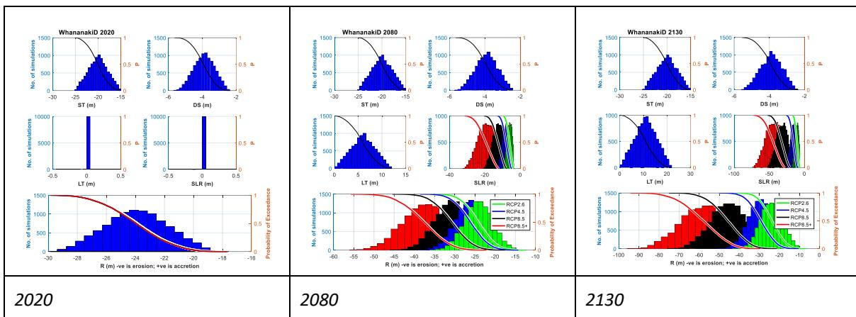
Figure 13-4 Histograms of parameter samples and the resultant shoreline distances for 2020, 2080 and 2130 timeframes for cell 13D
