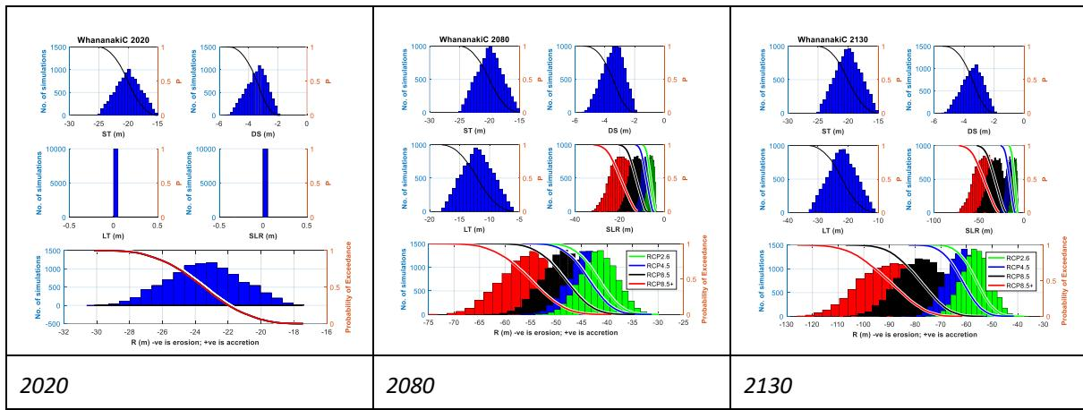
Figure 13-3 Histograms of parameter samples and the resultant shoreline distances for 2020, 2080 and 2130 timeframes for cell 13C
