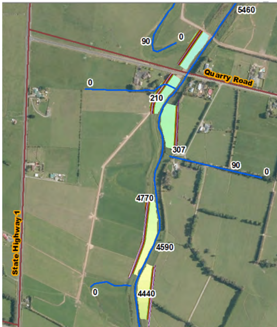
Figure 5-9: Benching along the Whangatane Spillway
