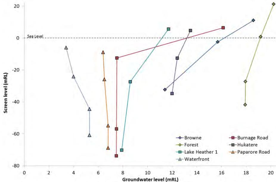
**Figure 5 Graph comparing the of top of screen and water level for multi-level piezometers**
