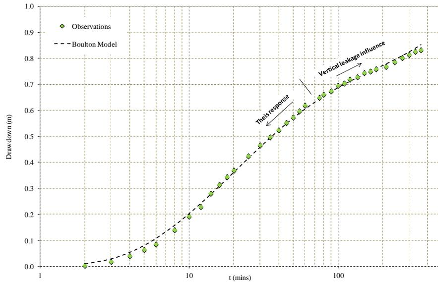
**Figure 6 Time-drawdown curve plot for the Ogle Drive aquifer test**
