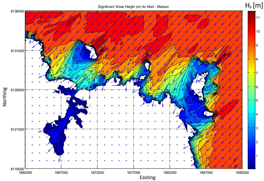
Figure Appendix B.7: SWAN model results for the Matauri model domain – Significant wave height and direction during a 100-year ARI storm from the Northeast
