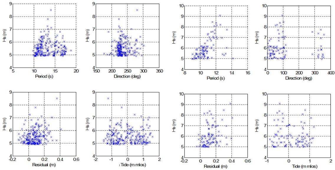
Figure 2.13: Storm peak characteristics for Ahipara (left) and Matauri (right) relating wave height to wave period, direction, non-tidal residual (storm surge) and tide
