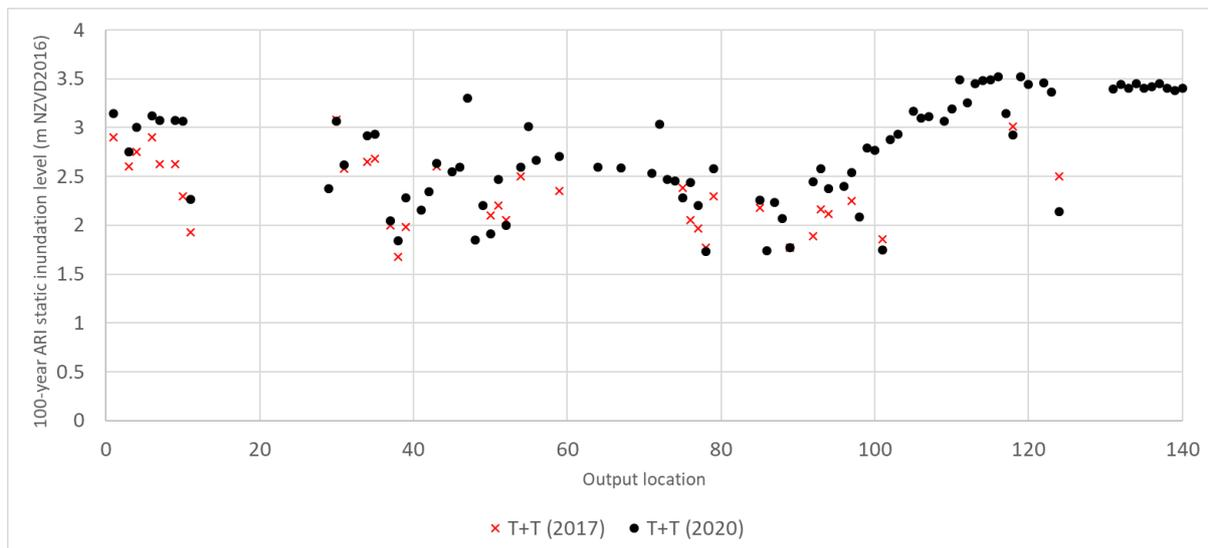
Figure 4.11: 100-year ARI static inundation levels derived by T+T (2017) and T+T (2020) for open coast sites
