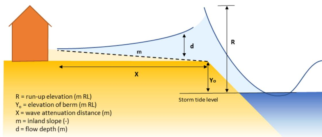
Figure 4.9: Run-up attenuation definition sketch (modified from Cox and Machemehl, 1986)
