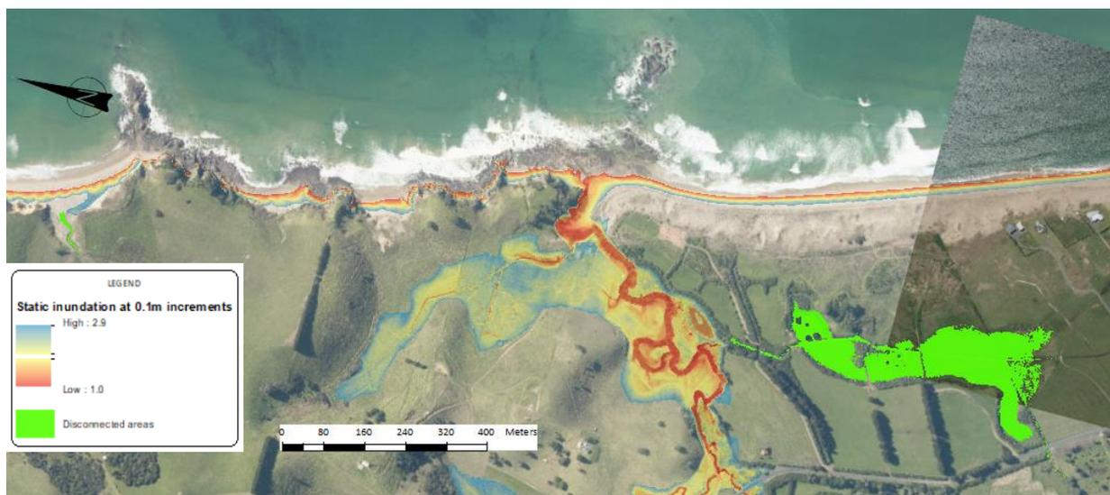
Figure 4.4: Example of inundation extents at 0.1 m increments at Pataua, with disconnected area shown for 2.9 m NZVD2016 level
