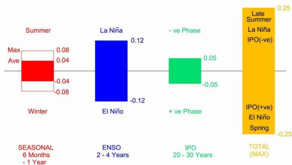
Figure 2.6: Variability in mean level of the sea due to climate cycles (source: Stephens and Bell, 2012)
