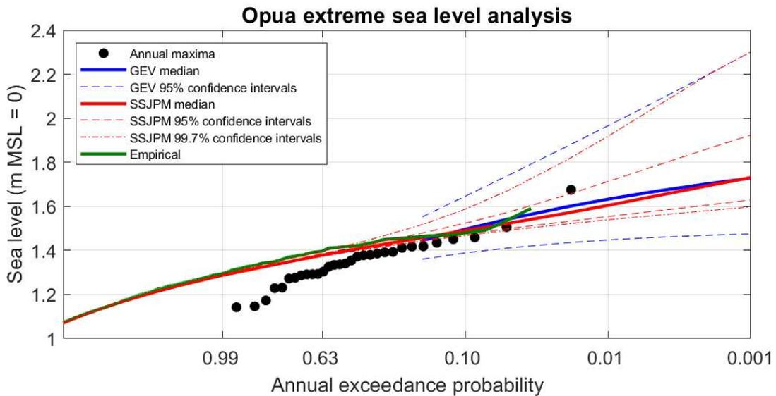
**Figure 4: Extreme sea level at Opua.** Elevations are plotted in metres relative to MSL = 0. They require a datum offset to convert them to a known datum such as OTP-64 (e.g., Table 2). The skew-surge joint-probability method (SSJPM) has been compared to the annual maxima (AM) plotted in their Gringorten (1963) plotting positions, a
