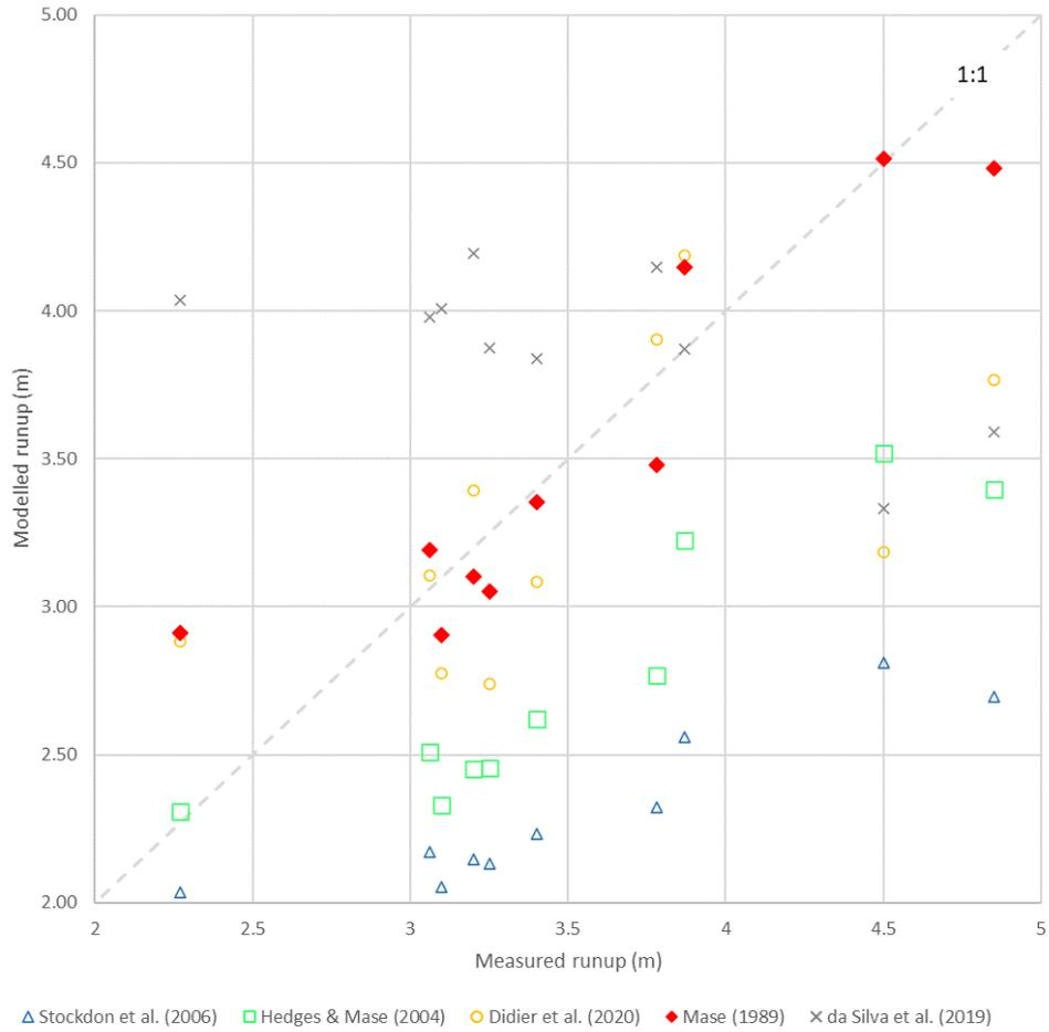
Figure 3.12: Plotted measured and modelled run-up
