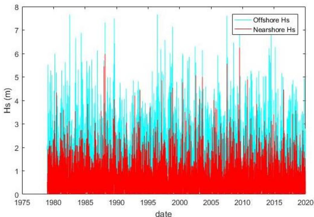
Figure 3.5: Example of offshore wave height timeseries and transformed nearshore wave height timeseries at Ruakaka
