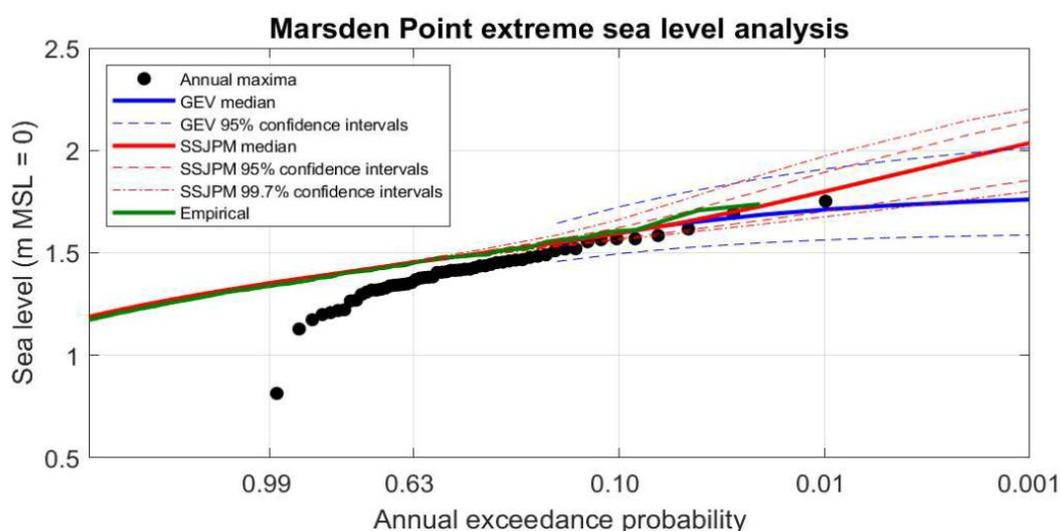
Figure 2.5: Extreme sea-level at Marsden Point relative to MSL = 0. The skew-surge joint-probability method (SSJPM) has been compared to the annual maxima (AM) plotted in their Gringorten (1963) plotting positions, a generalised extreme value distribution fitted to the AM, and an empirical distribution of the observed peak sea levels at high tide (source: NIWA, 2020)
