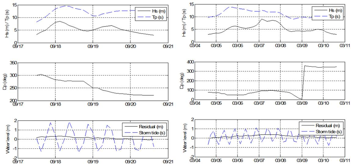
Figure 2.14: Time series of maximum storm on record for the Ahipara offshore site (September 2005) and for the Matauri site (March 1988)
