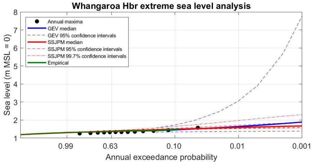
**Figure 5: Extreme sea level at Whangaroa.** Elevations are plotted in metres relative to MSL = 0. They require a datum offset to convert them to a known datum such as OTP-64 (e.g., Table 2). The skew-surge joint-probability method (SSJPM) has been compared to the annual maxima (AM) plotted in their Gringorten (1963) plotting positions, a generalised extreme-value distribution fitted to the AM, and an empirical distribution of the observed peak sea-levels at high tide. (e.g., Table 2).
