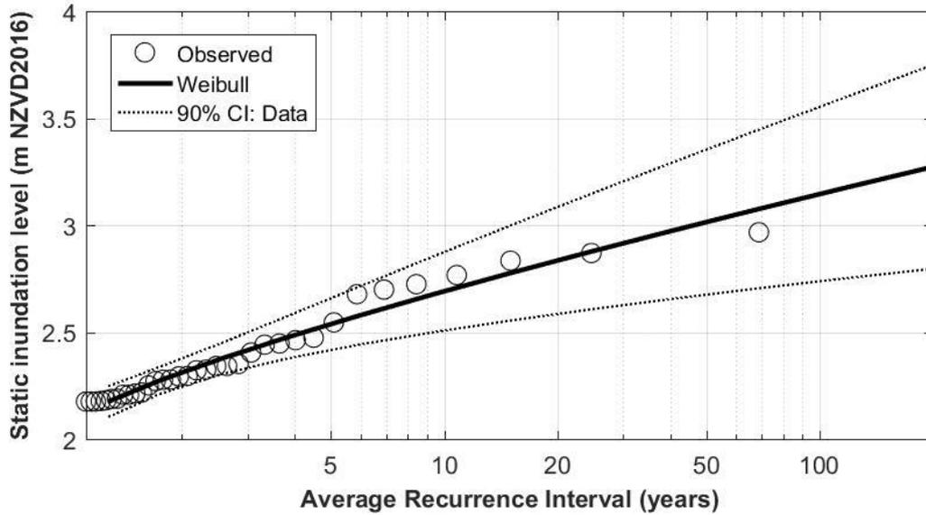
Figure 3.9: Example of extreme value analysis for static inundation level
