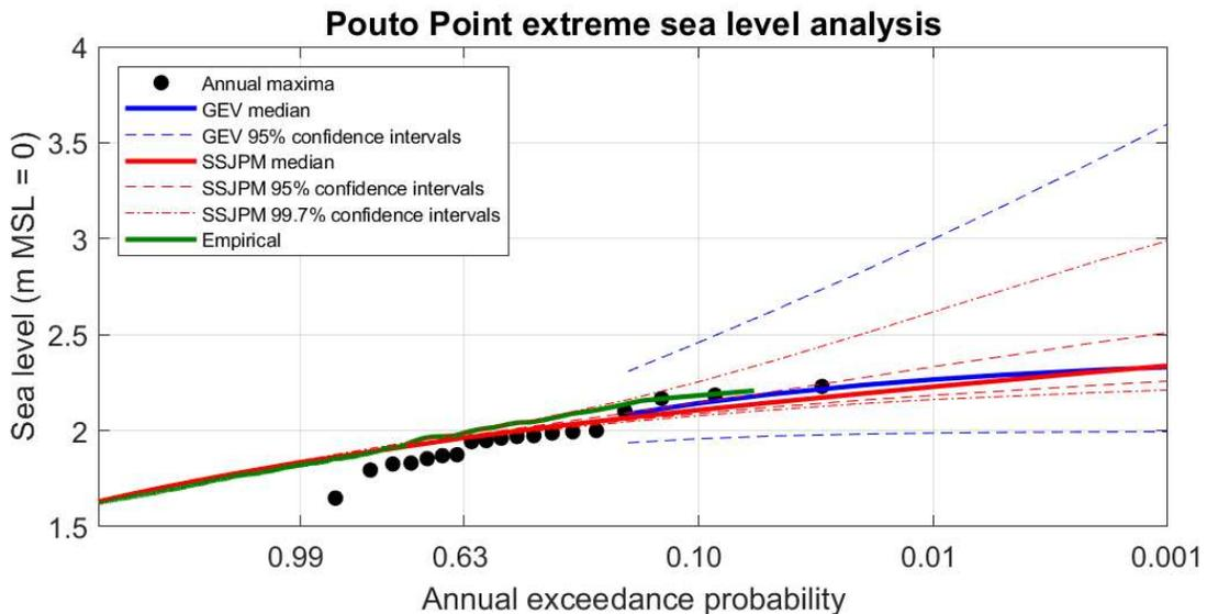
**Figure 2: Extreme sea level at Pouto Point.** Elevations are plotted in metres relative to MSL = 0. They require a datum offset to convert them to a known datum such as OTP-64 (e.g., Table 2). The skew-surge joint-probability method (SSJPM) has been compared to the annual maxima (AM) plotted in their Gringorten (1963) plotting positions,
