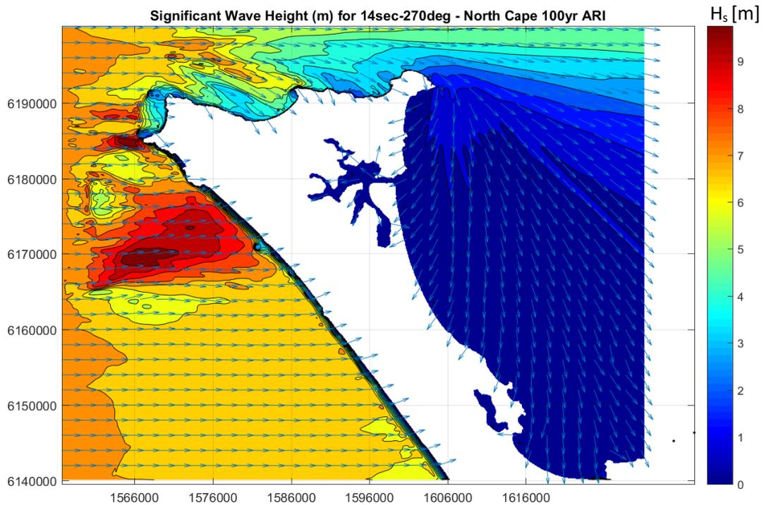
Figure Appendix B.4: SWAN model results for the North Cape domain – Significant wave height and direction during a 100-year ARI storm from the northeast
