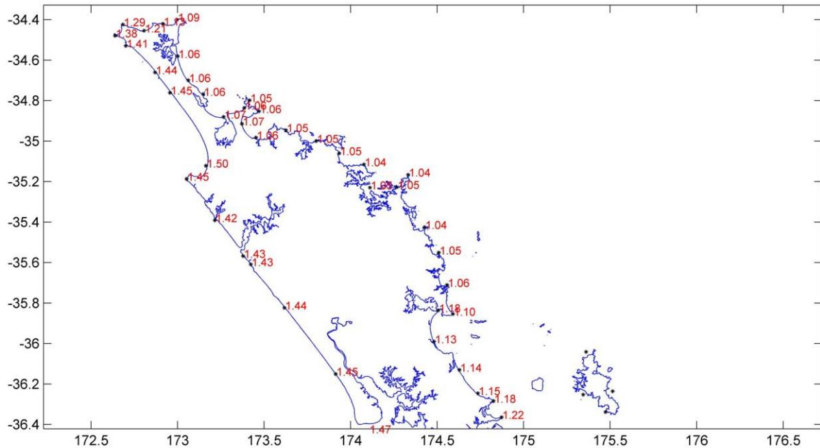
Figure 2.3: Plot of the mean high water springs level exceeded by 10% of tide (MHWS-10) level relative to MSL = 0 (Source: NIWA,2015)
