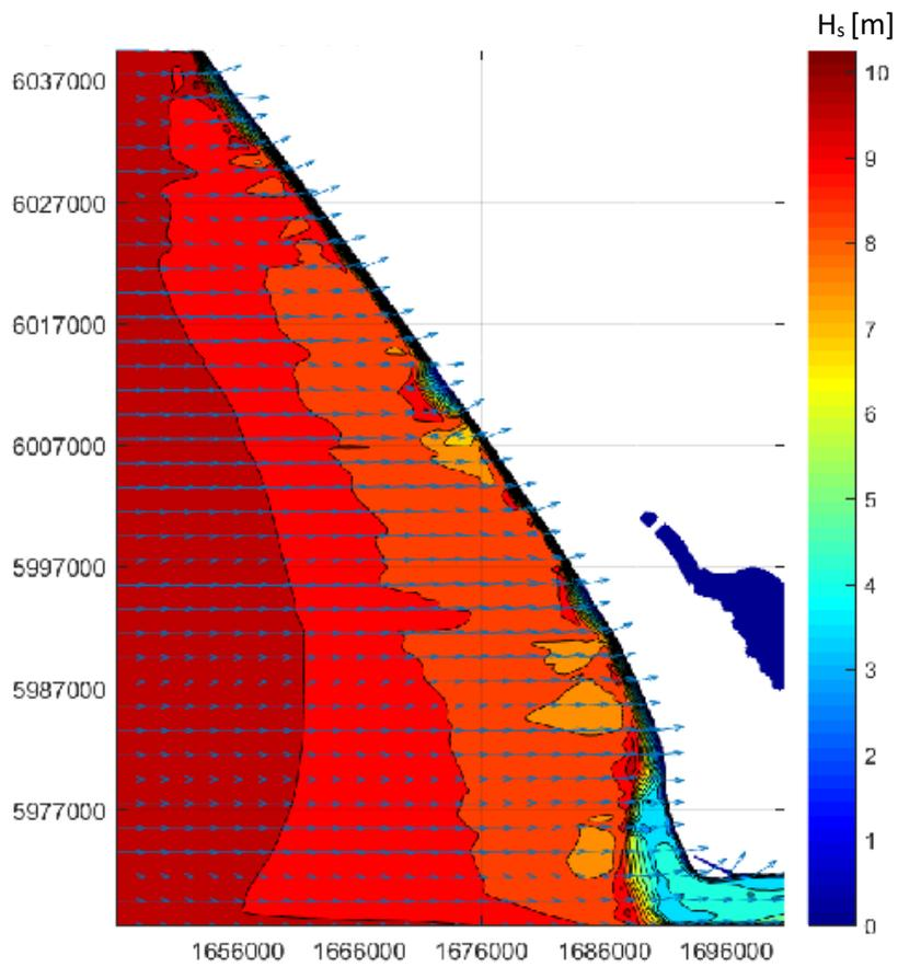
Figure Appendix B.2: SWAN model results for the South West Coast domain – Significant wave height and direction during a 100-year ARI storm from the west
