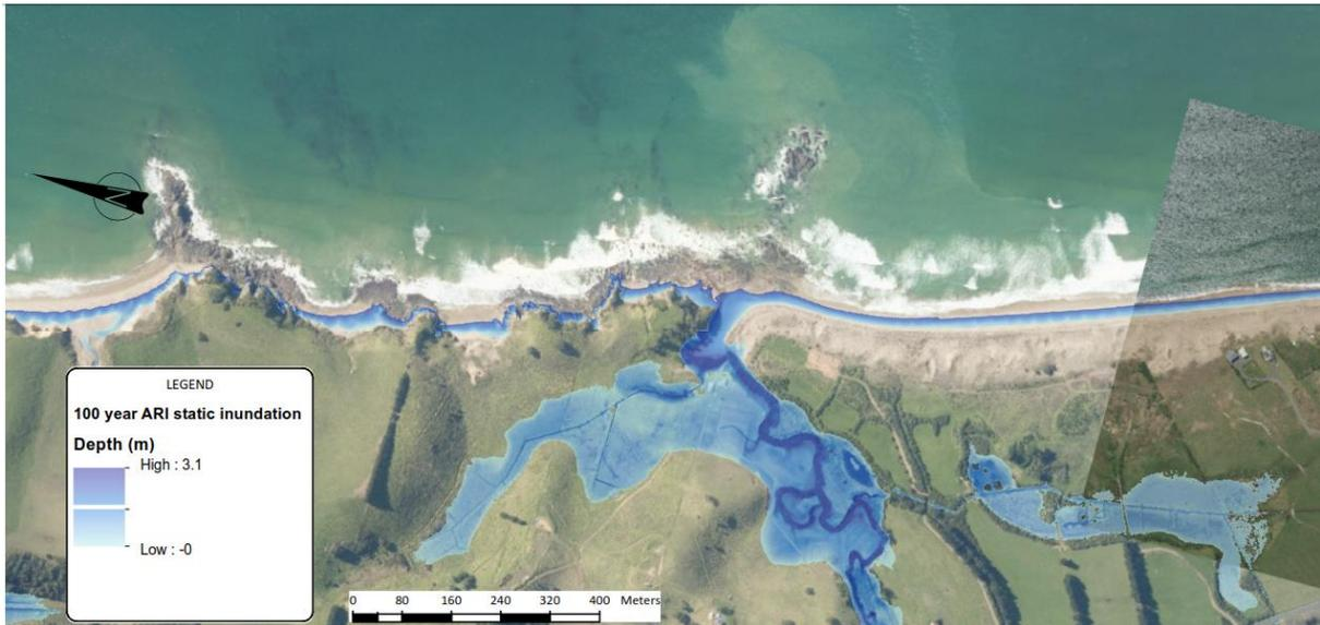
Figure 4.5: Example of inundation depths for a static inundation level of 2.9 m NZVD2016 at Pataua
