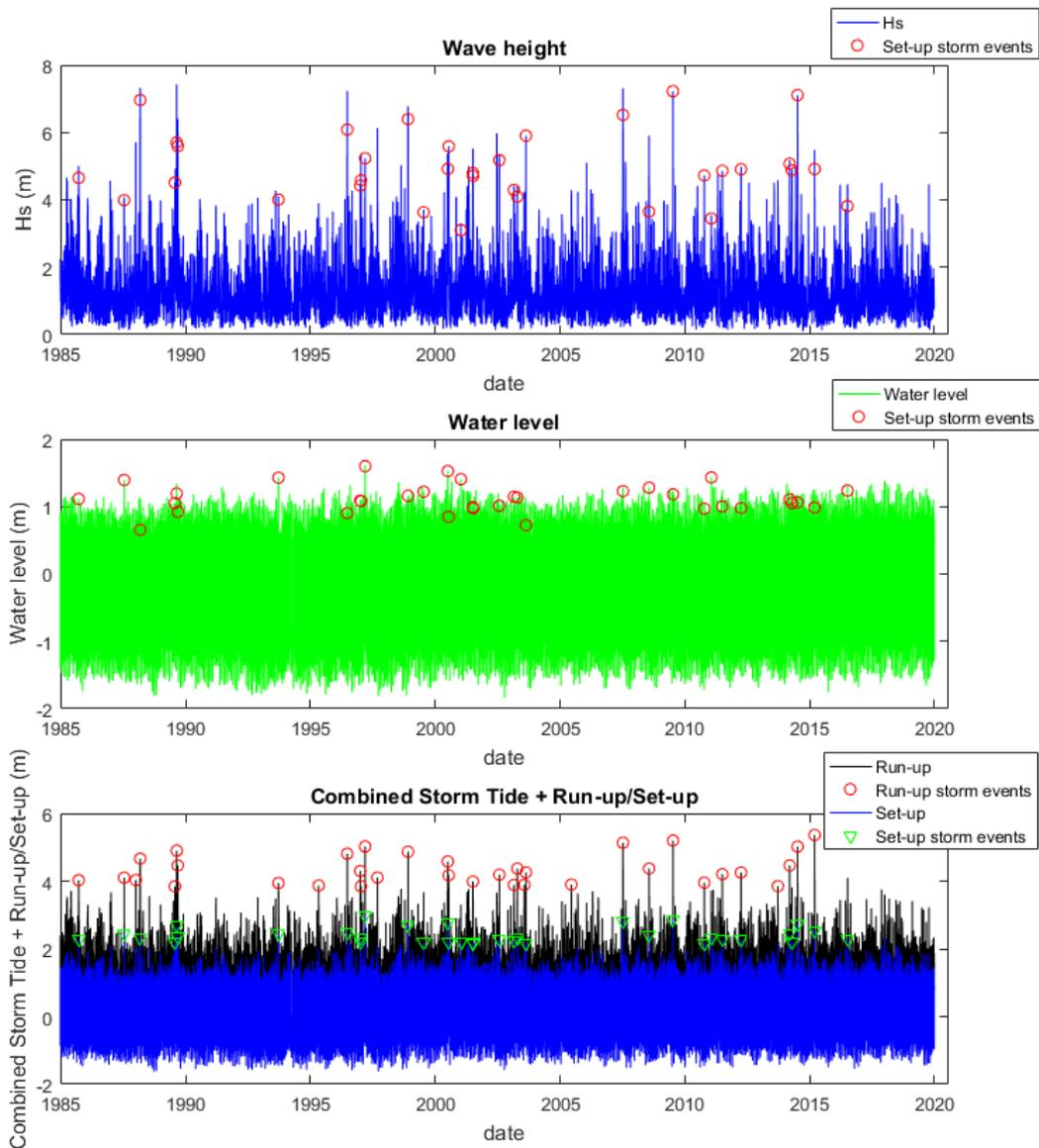
Figure 3.8: Timeseries of wave height (top panel), water level (middle panel) and combined water level + run-up and set-up (bottom panel) including identified extreme run-up and set-up events (shown as red circles and green triangles)
