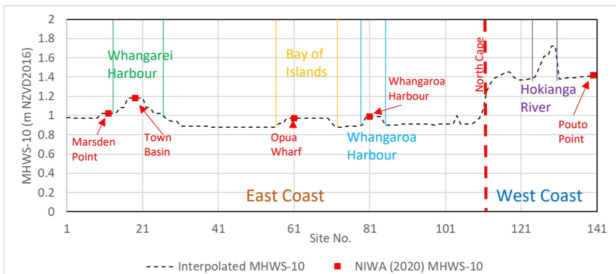
Figure 3.4: Rationalised MHWS-10 levels for output locations based on NIWA (2015) and LINZ (2020), including levels derived for tide gauges by NIWA (2020)
