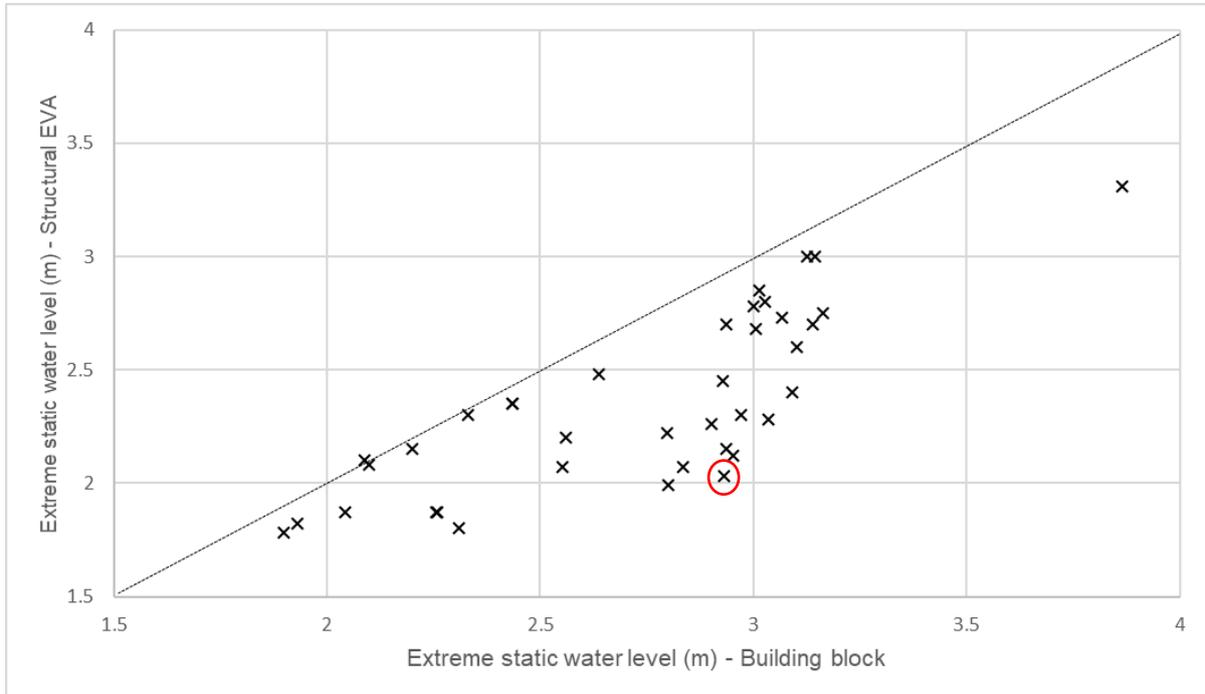
Figure 3.10: Comparison of extreme static water level calculated using the building block with the structural EVA approach based on T+T (2017)
