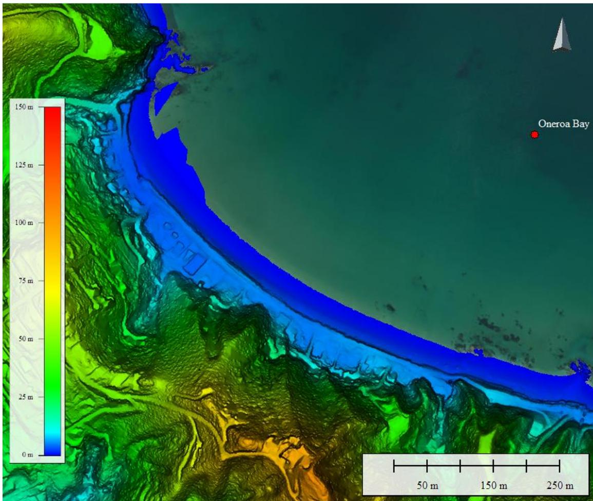
Figure 2.1: Example of 1 m DEM derived from 2019 LiDAR data for Oneroa Bay (Long Beach)
