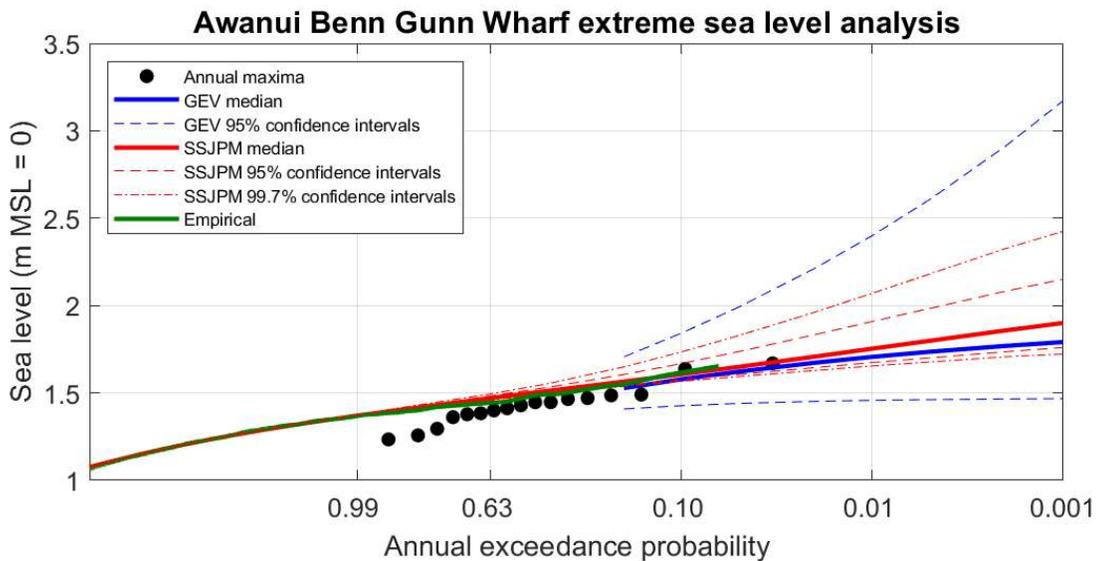
**Figure 6: Extreme sea level at Awanui Ben Gunn Wharf.** Elevations are plotted in metres relative to MSL = 0. They require a datum offset to convert them to a known datum such as OTP-64 (e.g., Table 2). The skew-surge joint-probability method (SSJPM) has been compared to the annual maxima (AM) plotted in their Gringorten (1963) plotting
