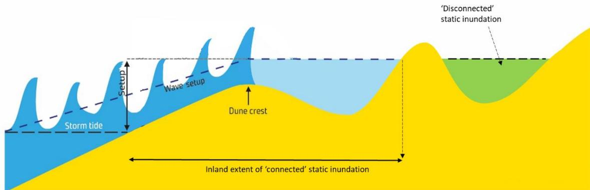
Figure 4.3: Connected and disconnected bathtub approach sketch
