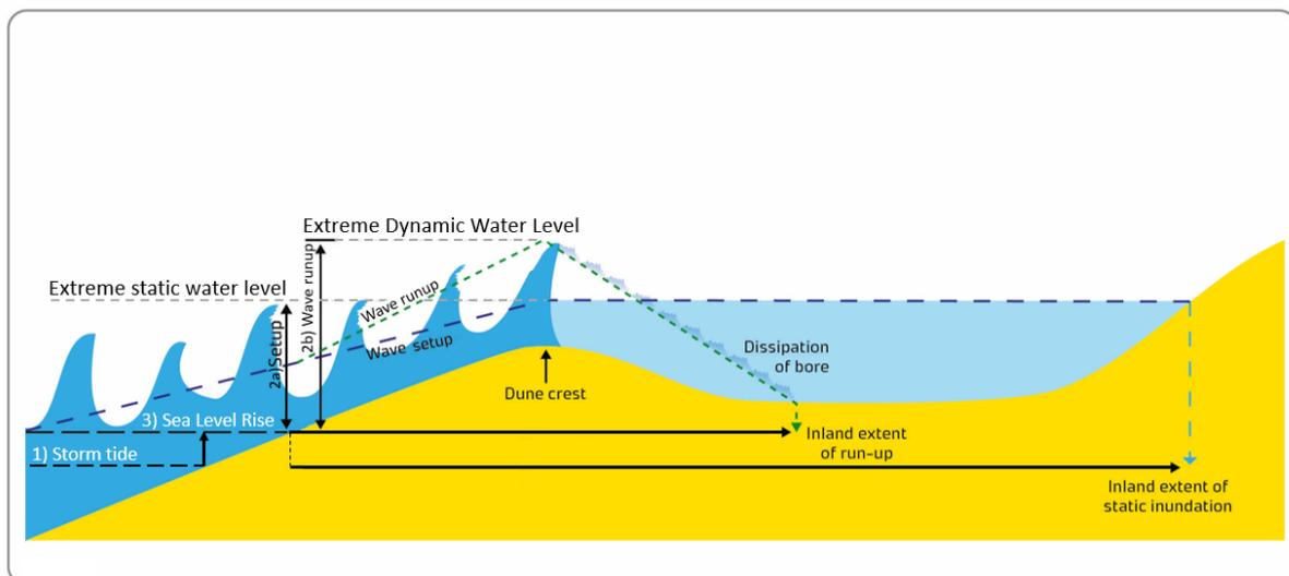
Figure 3.2: Schematisation of extreme water level components and combined extreme water levels
