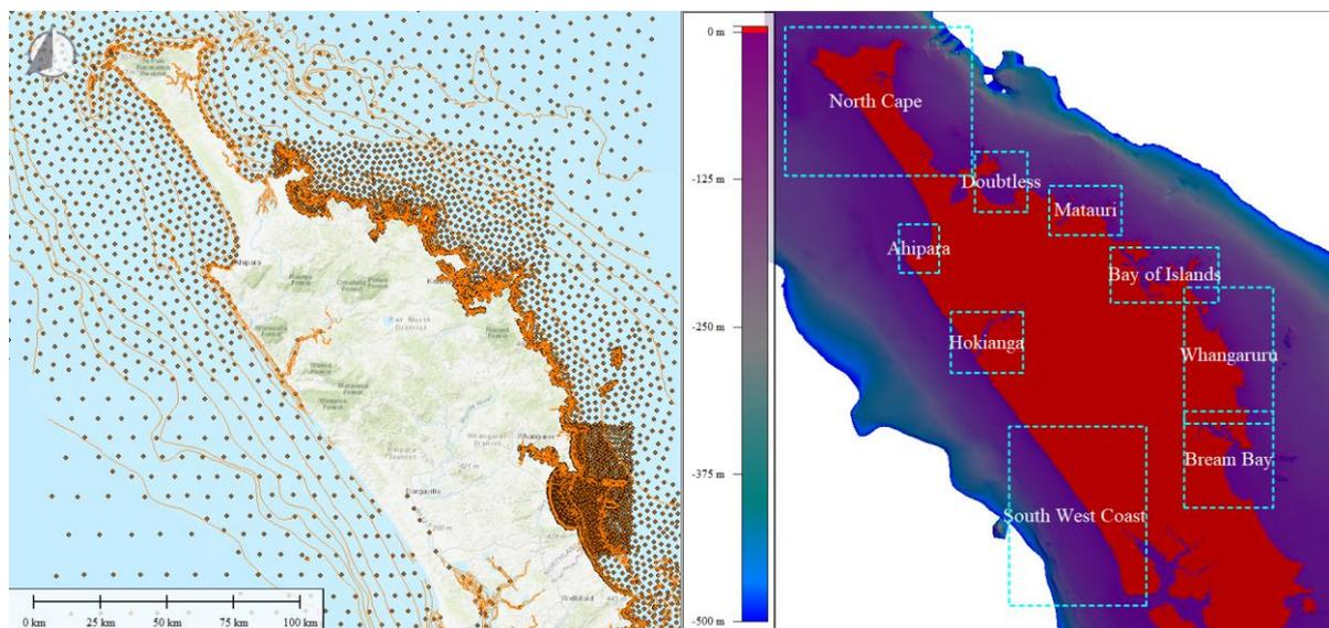
Figure Appendix B.1: Bathymetric contours and spot heights from LINZ database (A) and derived bathymetry map model (B) used to construct SWAN model domains (dashed boxes)
