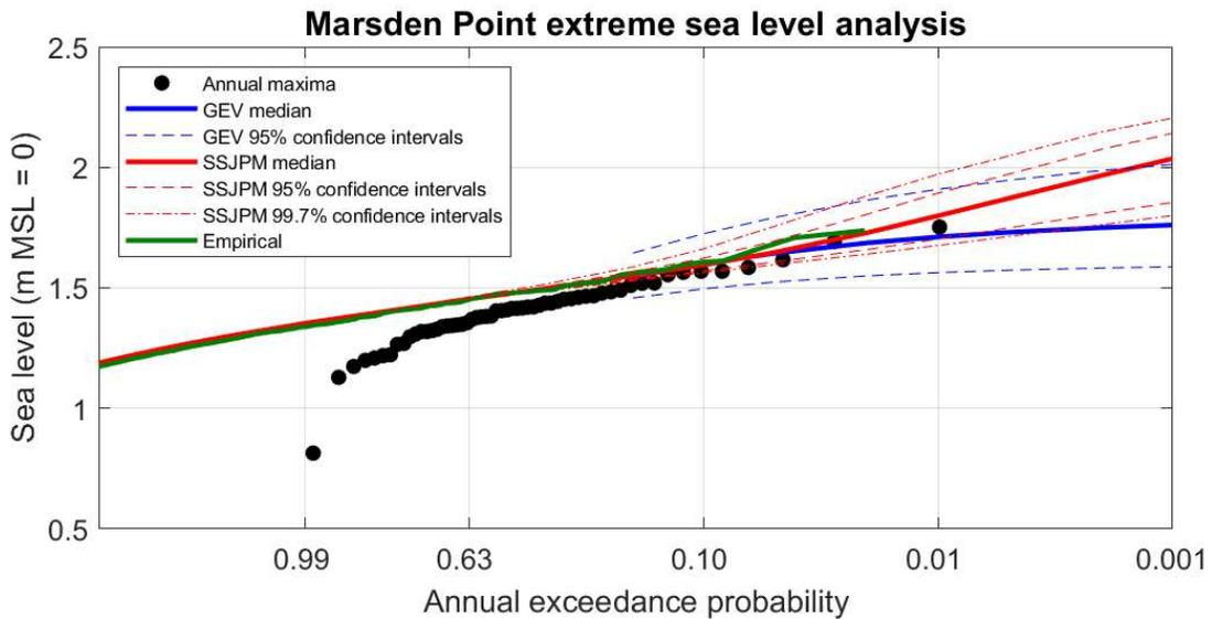
**Figure 1: Extreme sea level at Marsden Point.** Elevations are plotted in metres relative to MSL = 0. They require a datum offset to convert them to a known datum such as OTP-64 (e.g., Table 2). The skew-surge joint-probability method (SSJPM) has been compared to the annual maxima (AM) plotted in their Gringorten (1963) plotting positions, a generalised extreme-value distribution fitted to the AM, and an empirical distribution of the observed peak sea-levels at high tide.
