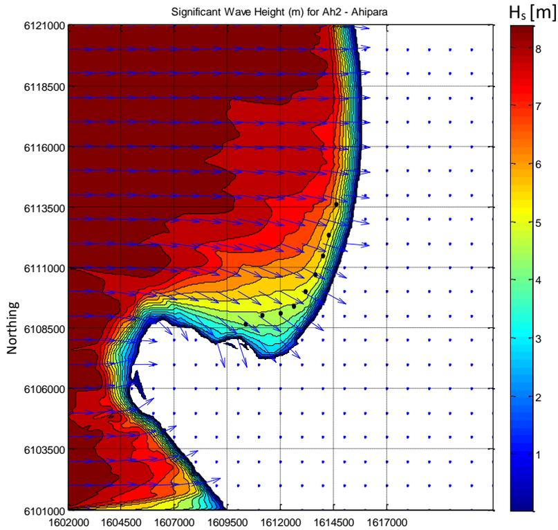
Figure Appendix B.3: SWAN model results for the Ahipara domain – Significant wave height and direction during a 100-year ARI storm from the west
