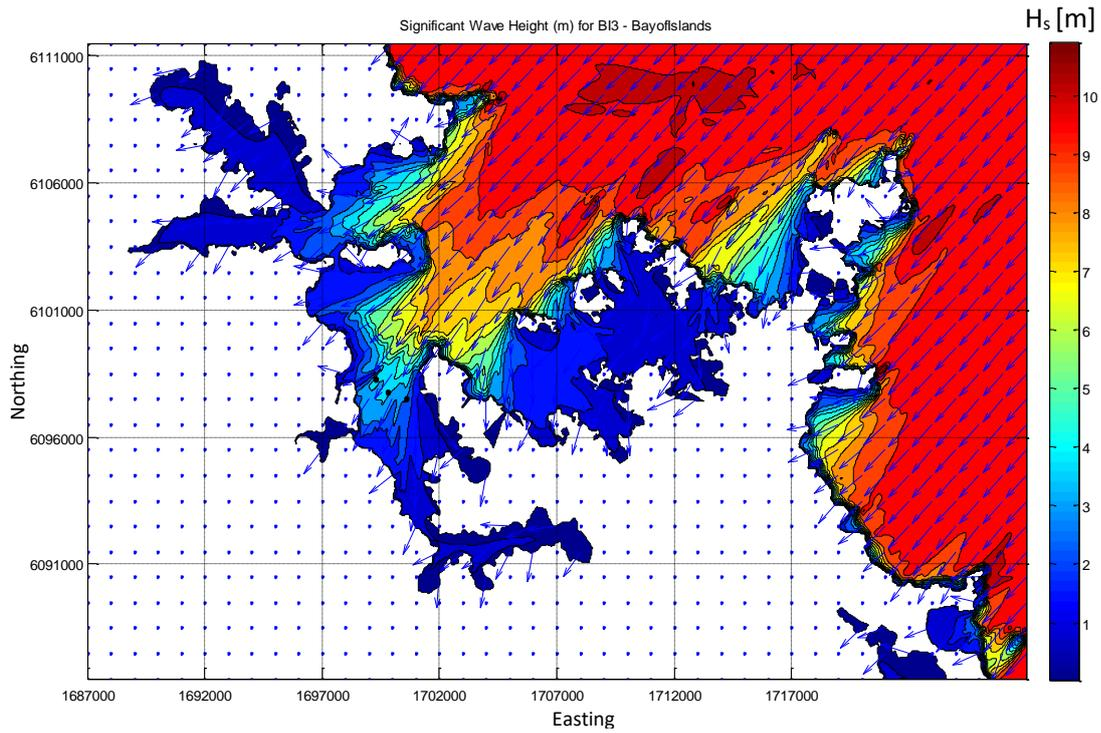
Figure Appendix B.6: SWAN model results for the Bay of Islands model domain – Significant wave height and direction during a 100-year ARI storm from the Northeast
