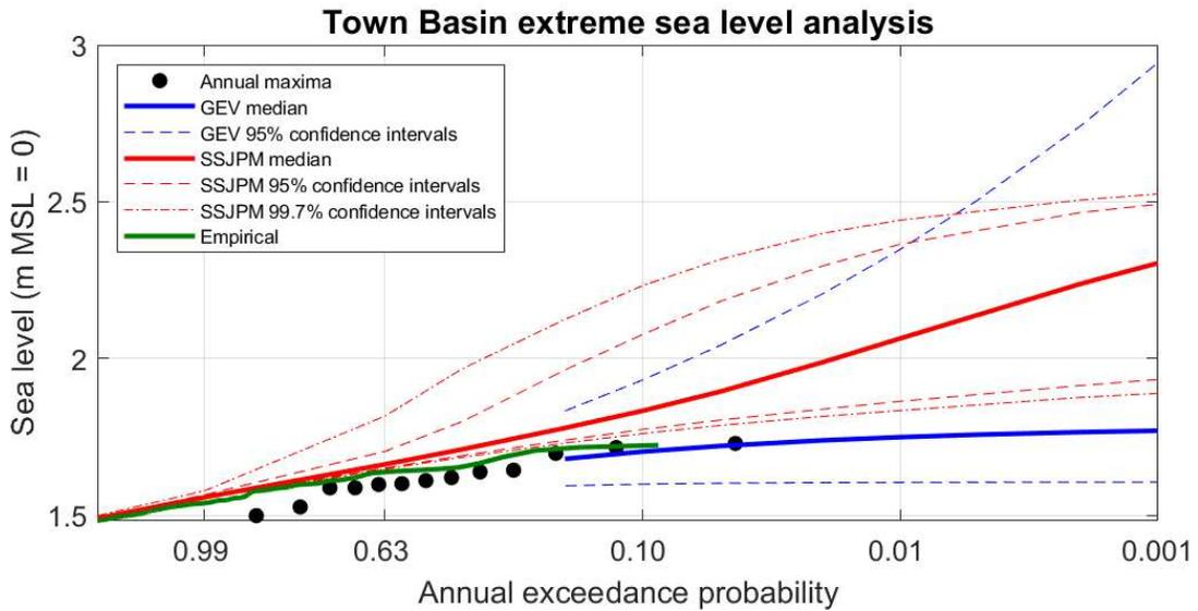
**Figure 3: Extreme sea level at Town Basin.** Elevations are plotted in metres relative to MSL = 0. They require a datum offset to convert them to a known datum such as OTP-64 (e.g., Table 2). The skew-surge joint-probability method (SSJPM) has been compared to the annual maxima (AM) plotted in their Gringorten (1963) plotting positions, a generalised extreme-value distribution fitted to the AM, and an empirical distribution of the observed peak sea-levels at high tide. (e.g., Table 2).
