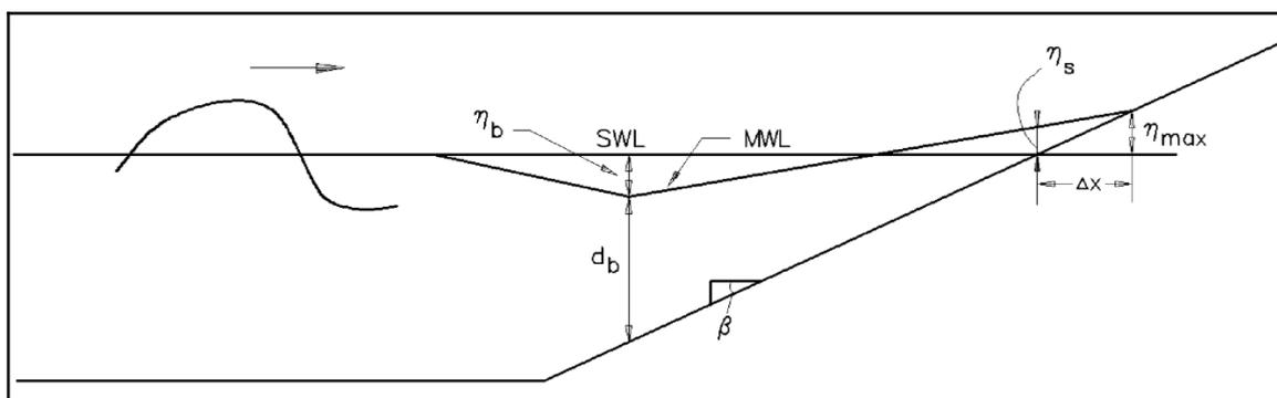
Figure 3.7: Wave set-up method (source: USACE, 2006)
