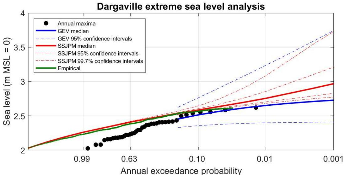
**Figure 7: Extreme sea level at Dargaville.** Elevations are plotted in metres relative to MSL = 0. They require a datum offset to convert them to a known datum such as OTP-64 (e.g., Table 2). The skew-surge joint-probability method (SSJPM) has been compared to the annual maxima (AM) plotted in their Gringorten (1963) plotting positions, a generalised extreme-value distribution fitted to the AM, and an empirical distribution of the observed peak sea-levels at high tide. (e.g., Table 2).
