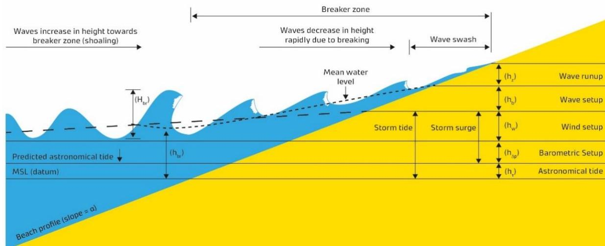
Figure 2.2: Key components that determine water level
