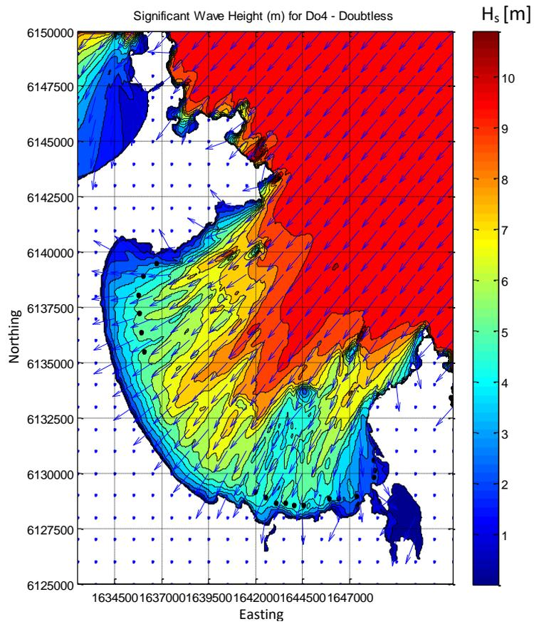
Figure Appendix B.5: SWAN model results for the Doubtless model domain – Significant wave height and direction during a 100-year ARI storm from the northeast
