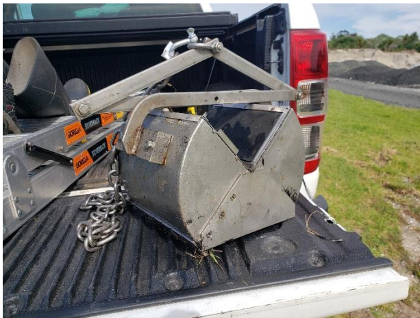
Photo 9: Ponar dredge used to collect sediment samples at Site 5 and 6 in the main settlement pond.
