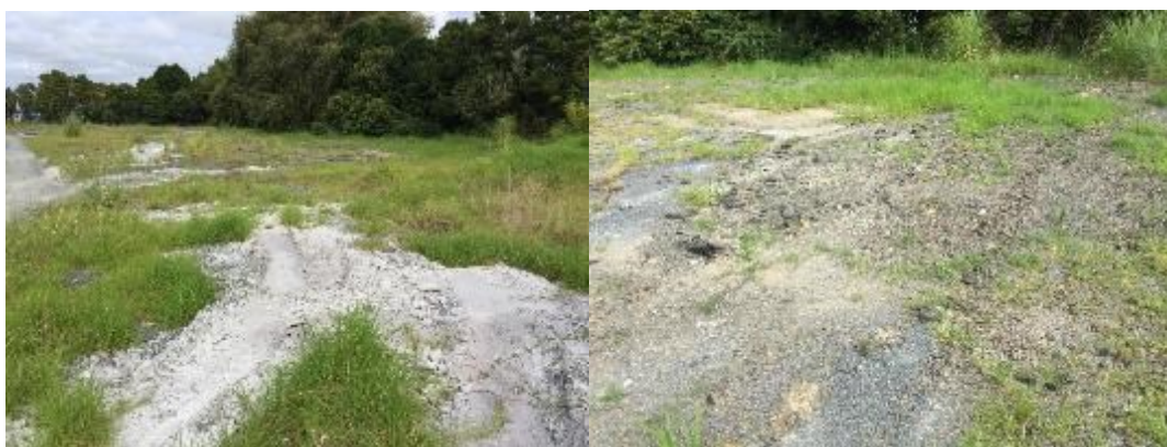
Photographs 2 & 3: Waste concrete and bitumen/gravel fill over the northern portion of the site
