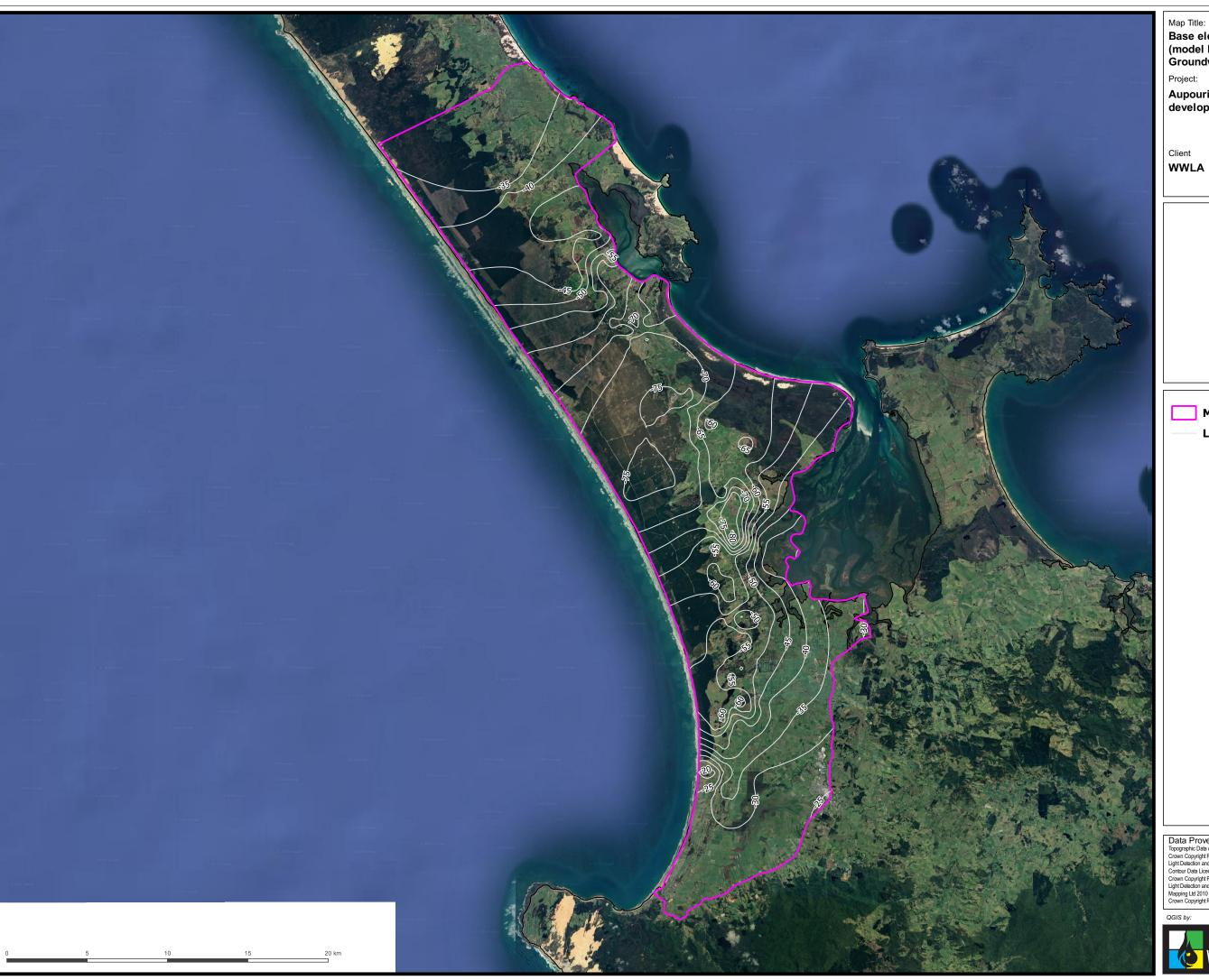
Base elevation the upper shellbed (model layer 4) in Aupouri Aquifer Groundwater Model
