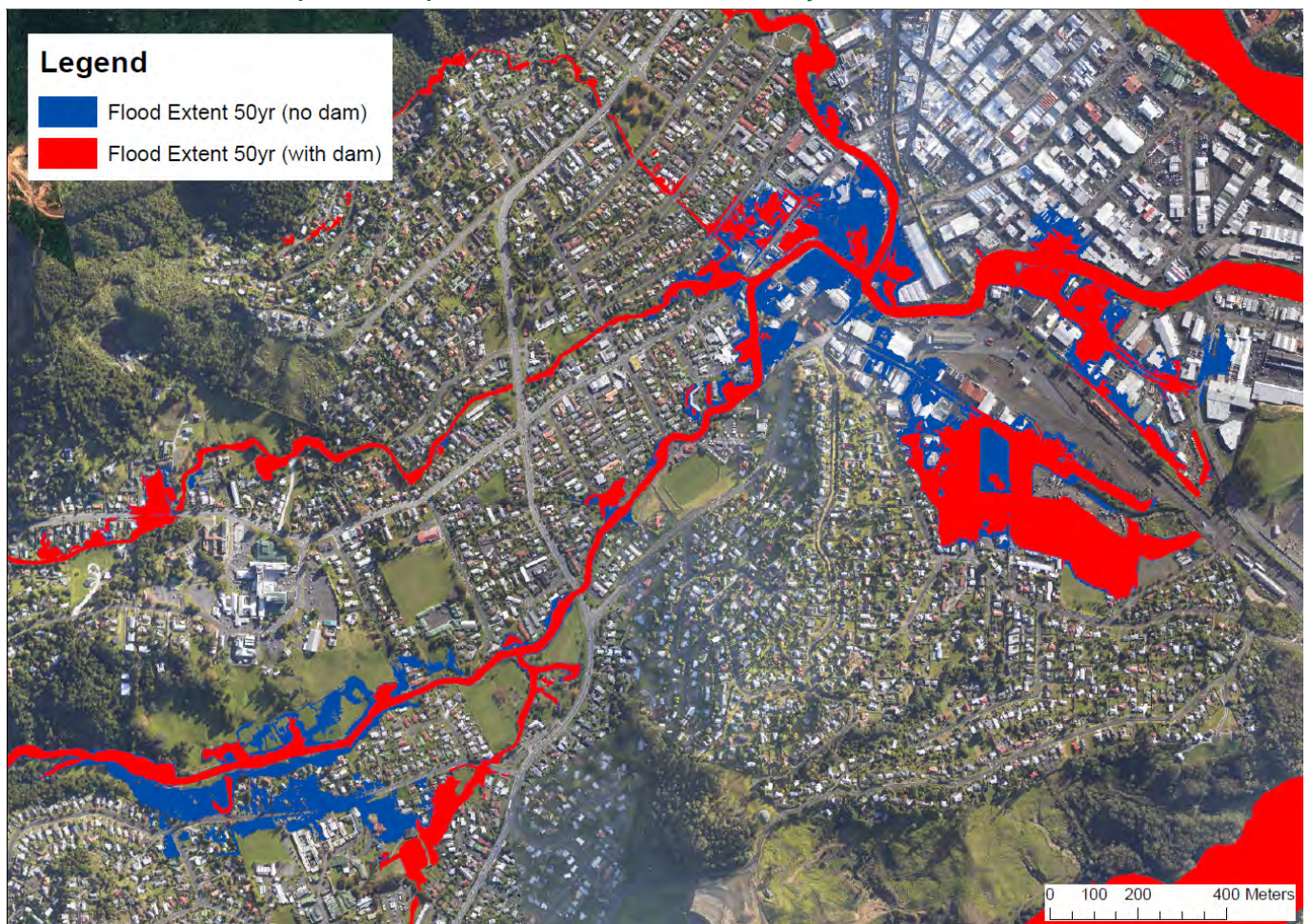
Impact of the 'Hopua te Nihotetea' detention dam of the 1:50yr flood extent in the CBD
