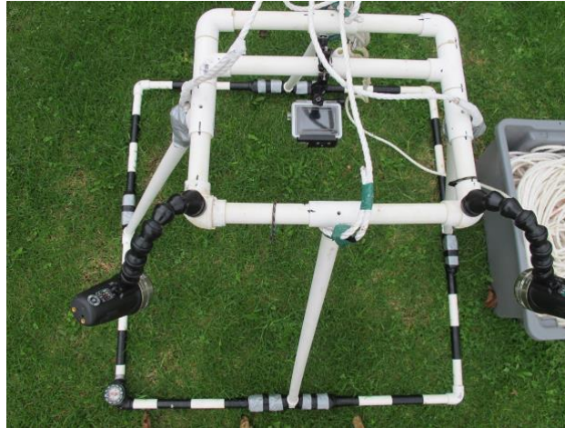
Figure 1 The GoPro drop camera quadrat apparatus used for the field survey
