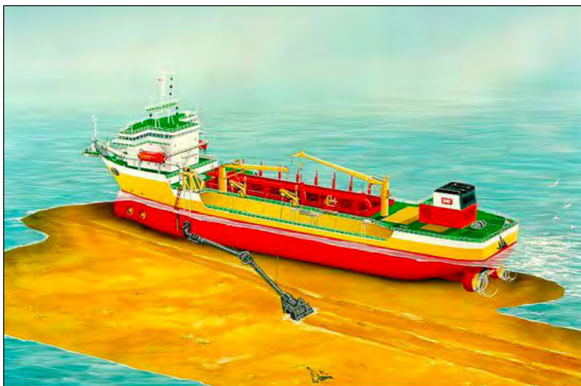
Figure 1.5.8.1: Example of a TSHD 23
