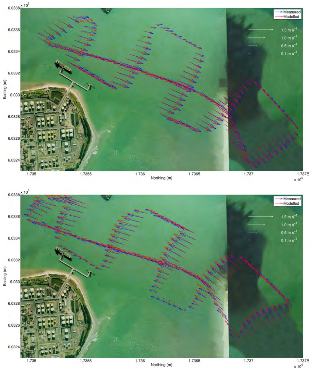
Figure 6.8 Modelled (Delft3D) and measured velocity comparisons within Zone A (Figure 5.2) for the ebb (upper) and flood (lower) tidal stages.
