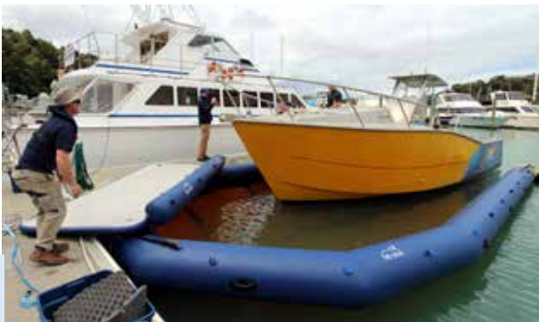
PHOTO: Northland Regional Council has been sharing knowledge with other local authorities, with a training exercise showing how to deploy and use a portable, inflatable vessel quarantine facility (VQF).
