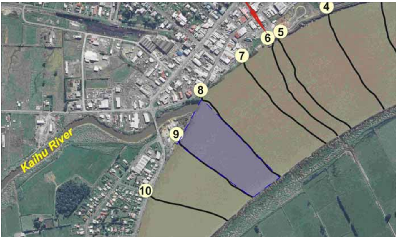
Figure 1: Control volume for junction analysis
