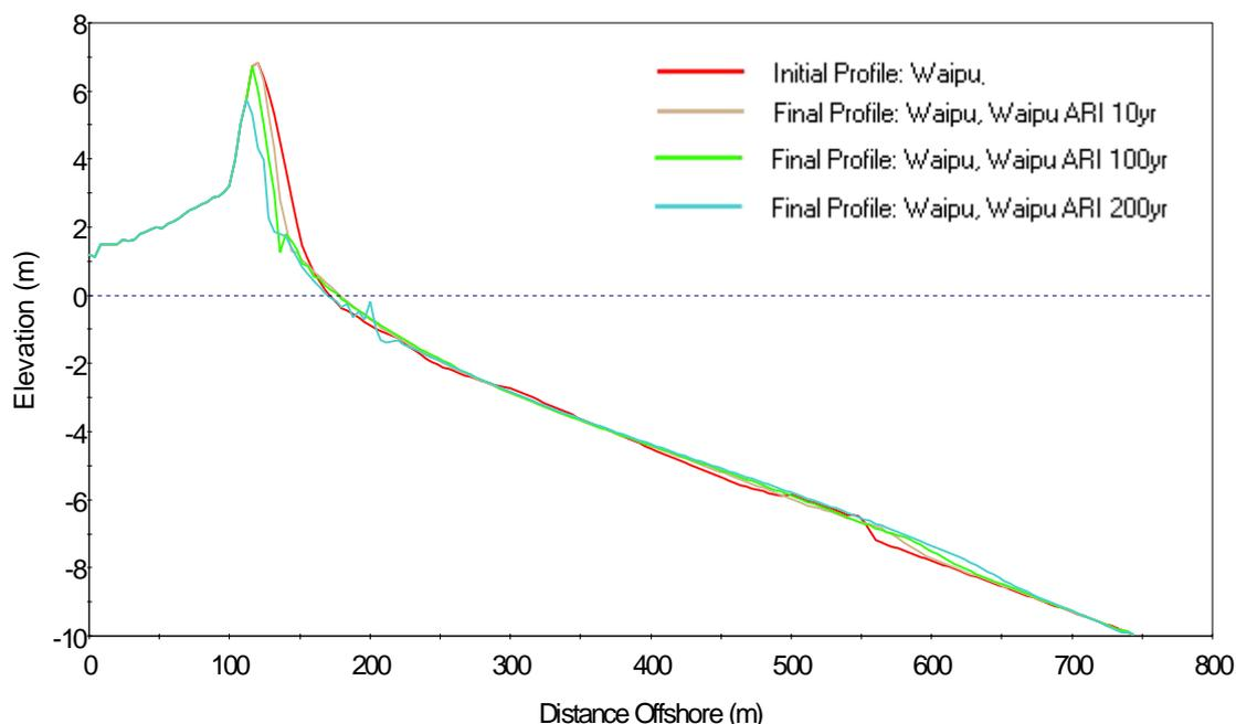
Figure 4-6 Example SBEACH results for Waipu Cove
