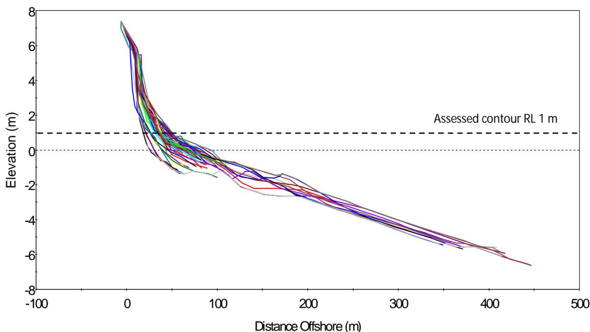
Figure 4-7 Example beach profiles for Waipu Cove
