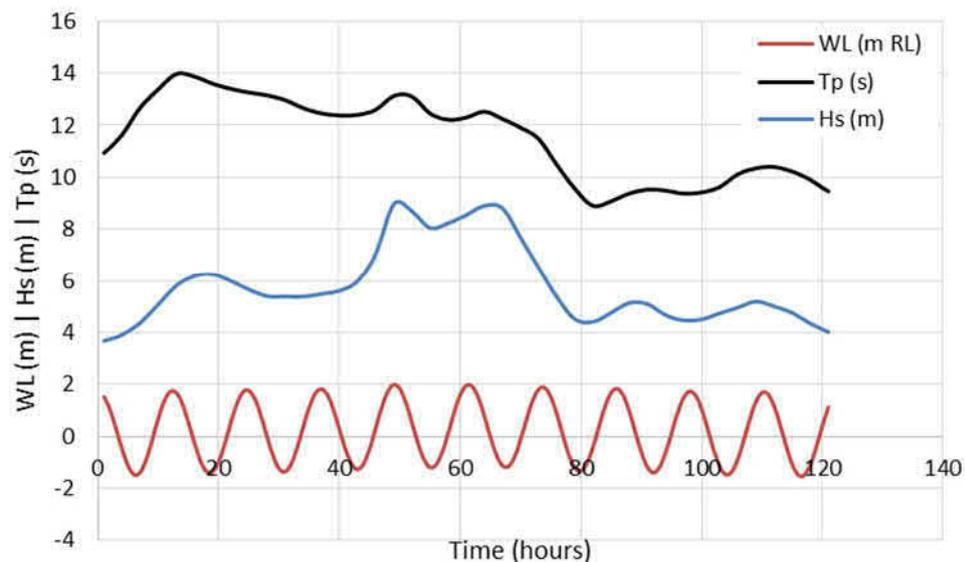
Figure B-1 Example 100 year ARI synthetic design storm for the west coast
