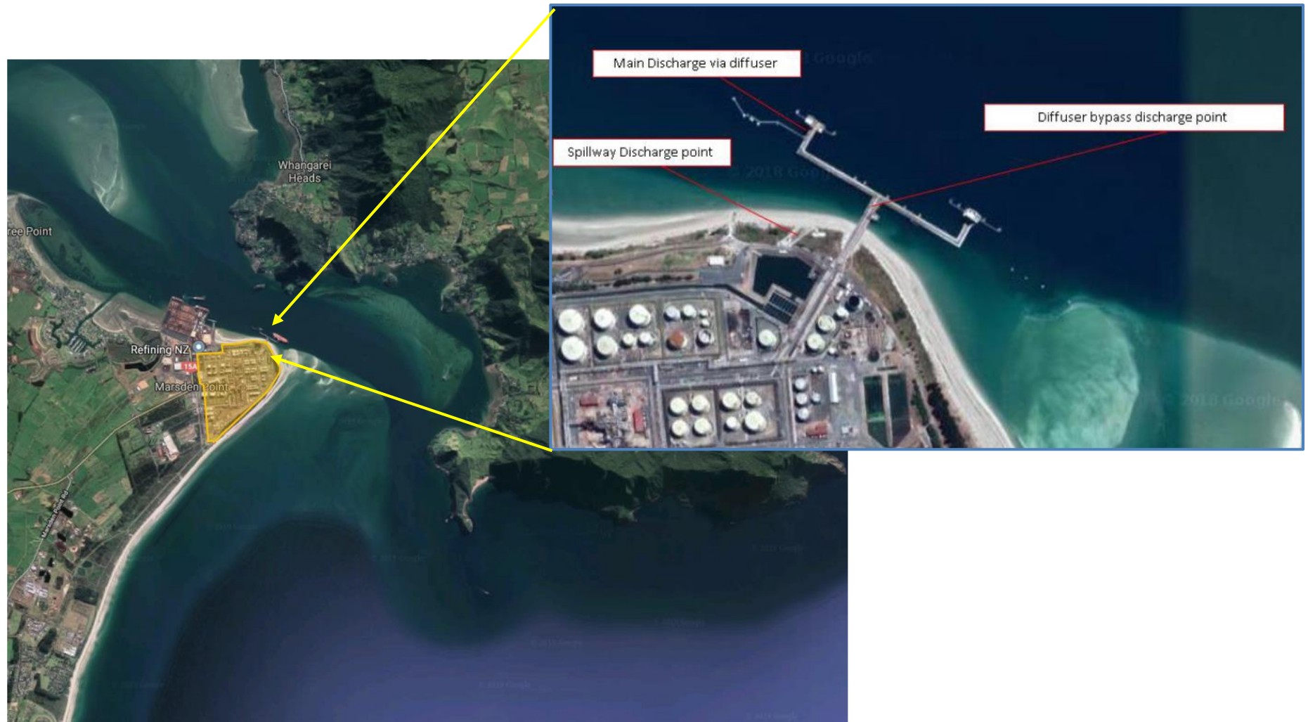
Figure 1. Aerial view of the extent (shown in yellow) of Refining New Zealand's Marsden Point refinery sited at the Whangarei Harbour entrance. Inset: Locations of the refinery's three possible marine discharge points.
