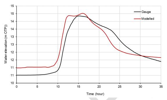
FIGURE 3-8 MODELLED AND GAUGED LEVELS AT OTAIKA RIVER AT KAY - 2011 FLOOD EVENT
