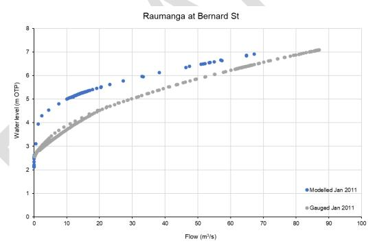
FIGURE 3-11 MODELLED AND GAUGED RATING CURVE COMPARISON AT BERNARD ST
