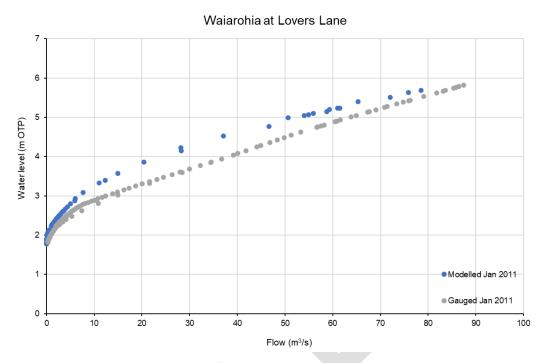
FIGURE 3-10 MODELLED AND GAUGED RATING CURVE COMPARISON AT LOVERS LANE GAUGE
