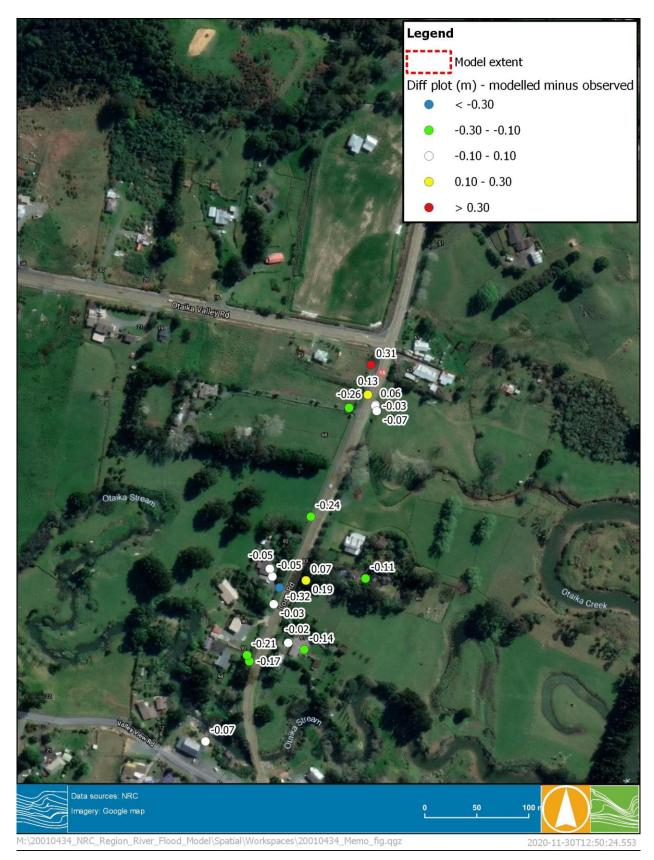
FIGURE 3-15 COMPARISON BETWEEN MODELLED FLOOD LEVEL AND SURVEY FLOOD LEVEL – JANUARY 2011 EVENT (EAST OF OTAIKA VALLEY RD)
