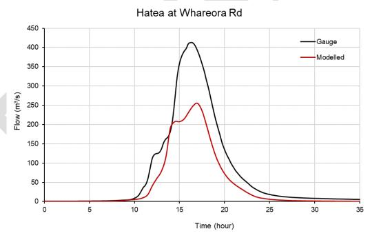
FIGURE 3-1 MODELLED AND GAUGED FLOW AT HATEA RIVER AT WHAREORA RD - 2011 FLOOD EVENT
