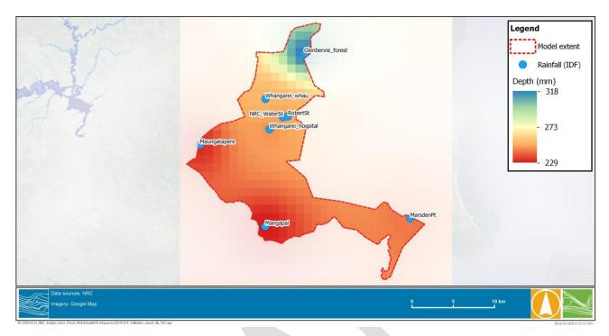
FIGURE 4-1 EXAMPLE OF DESIGN RAINFALL GRID (12-HOUR, 1% AEP RAINFALL) FOR M01
