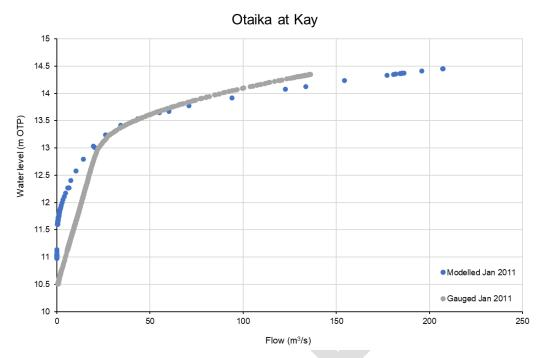
FIGURE 3-12 MODELLED AND GAUGED RATING CURVE COMPARISON AT KAY
