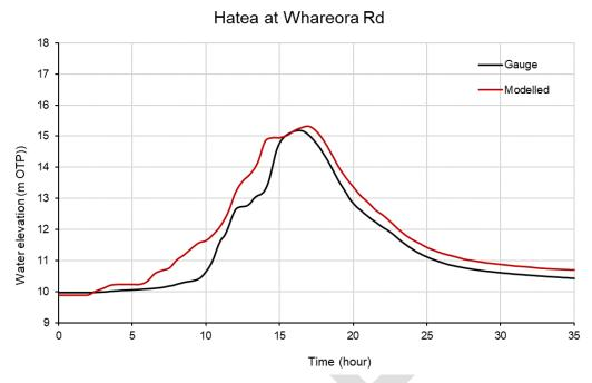
FIGURE 3-2 MODELLED AND GAUGED WATER LEVELS AT HATEA RIVER AT WHAREORA RD – 2011 FLOOD EVENT
