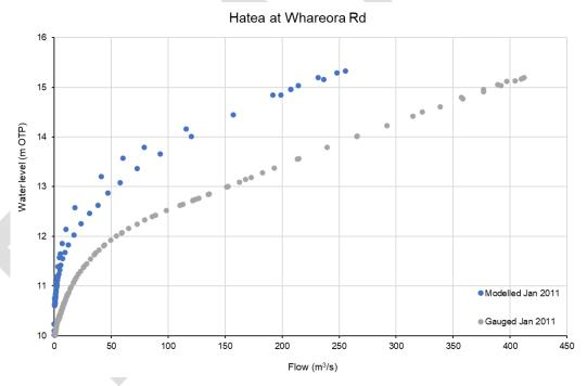
FIGURE 3-9 MODELLED AND GAUGED RATING CURVE COMPARISON AT WHAREORA RD GAUGE
