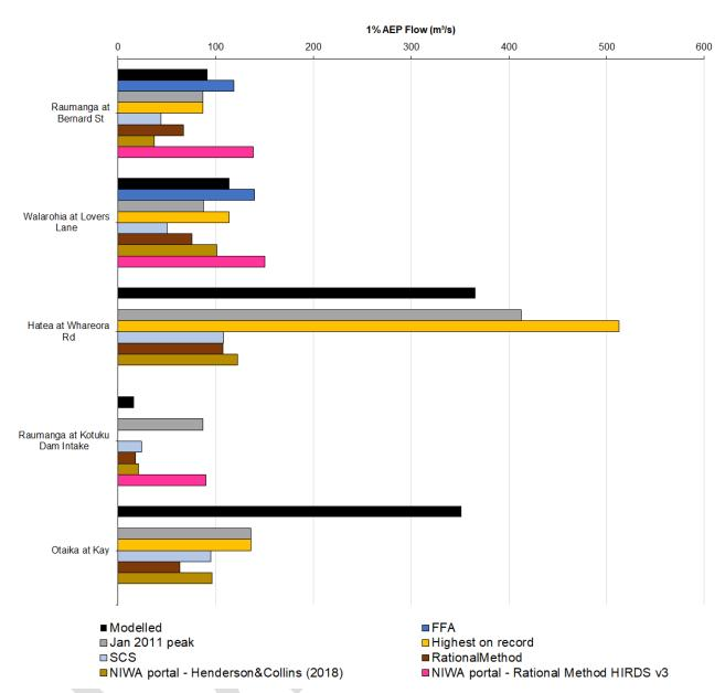
FIGURE 6-3 VERIFICATION OF DESIGN MODELLING RESULTS AGAINST HYDROLOGICAL ESTIMATES
