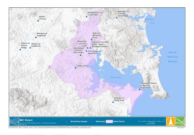
FIGURE 6-1 AVAILABLE STREAMFLOW GAUGES WITHIN WHANGAREI CATCHMENT
