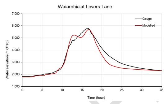
FIGURE 3-4 MODELLED AND GAUGED WATER LEVELS AT WAIAROHIA RIVER AT LOVERS LANE – 2011 FLOOD EVENT
