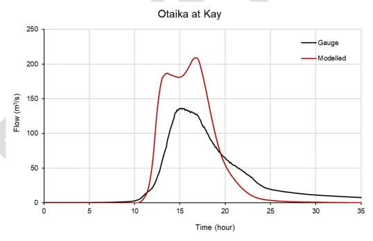
FIGURE 3-7 MODELLED AND GAUGED FLOWS FOR OTAIKA RIVER AT KAY - 2011 FLOOD EVENT
