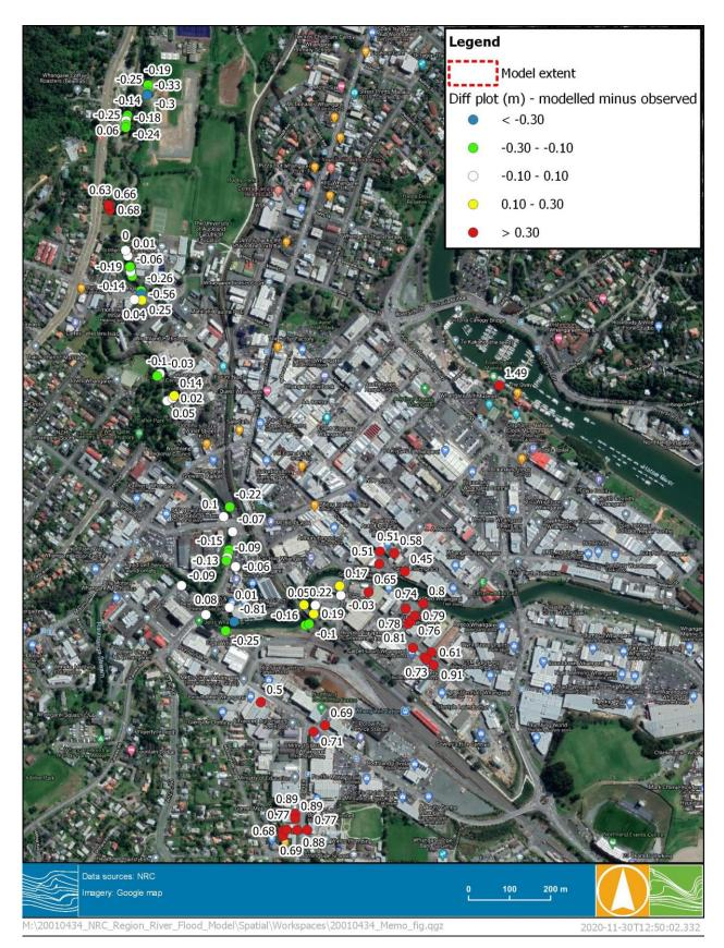
FIGURE 3-14 COMPARISON BETWEEN MODELLED FLOOD LEVEL AND SURVEY FLOOD LEVEL – JANUARY 2011 EVENT (TOWNSHIP OF WHANGAREI)
