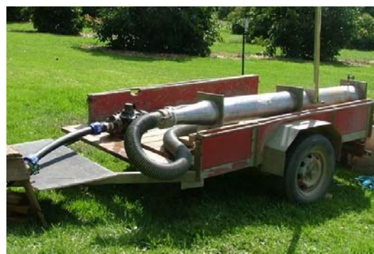
Orifice weir used for pump testing.
