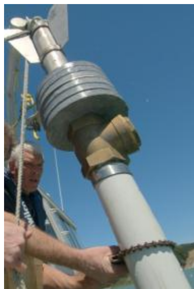
Gravity corer being deployed to collect sediment cores
