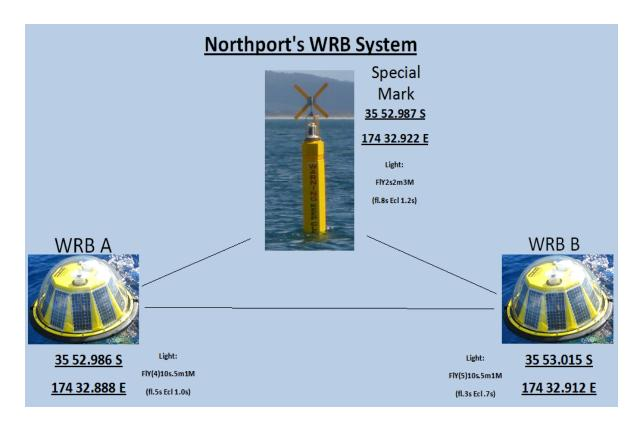
The yellow Special Mark Buoy is positioned to the north of the two Wave Rider Buoys at an equal distance from both. The Special Mark Buoy is deployed to indicate the position of the two smaller Wave Rider Buoys and is higher and more visible than the Wave Rider Buoys which sit very low in the water.
