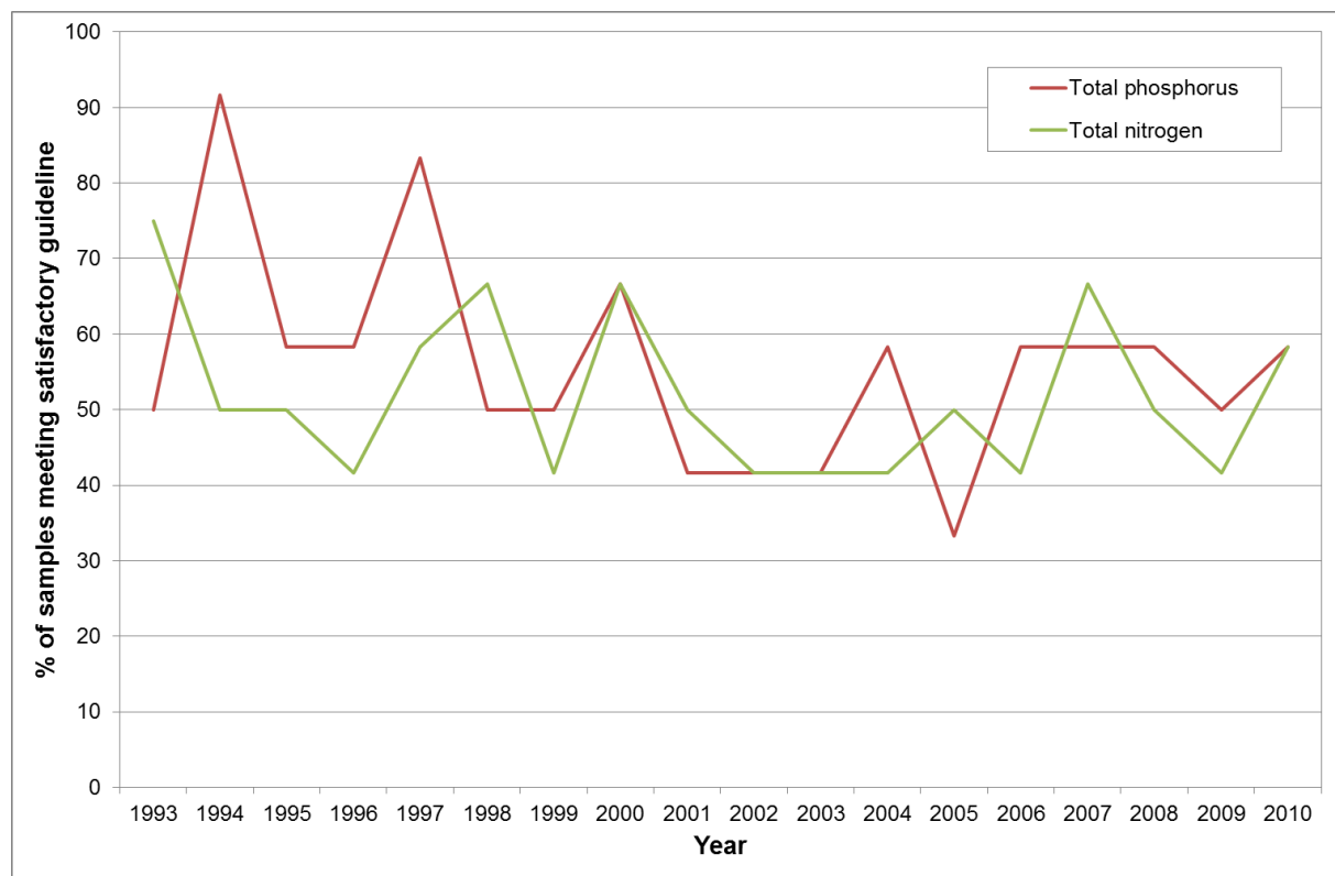
Figure 4: Percentage of samples at Waitetuna River site meeting Environment Waikato's "satisfactory" guidelines for total nitrogen and total phosphorus.
