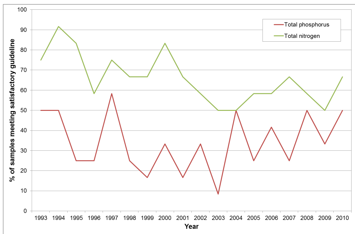
Figure 2: Percentage of samples at Ohautira Stream site meeting Environment Waikato's "satisfactory" guidelines for total nitrogen and total phosphorus.
