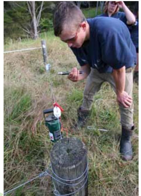
Hagan Skelton, from Tauraroa Area School, uses a homemade electric fence tester to locate a fault.
