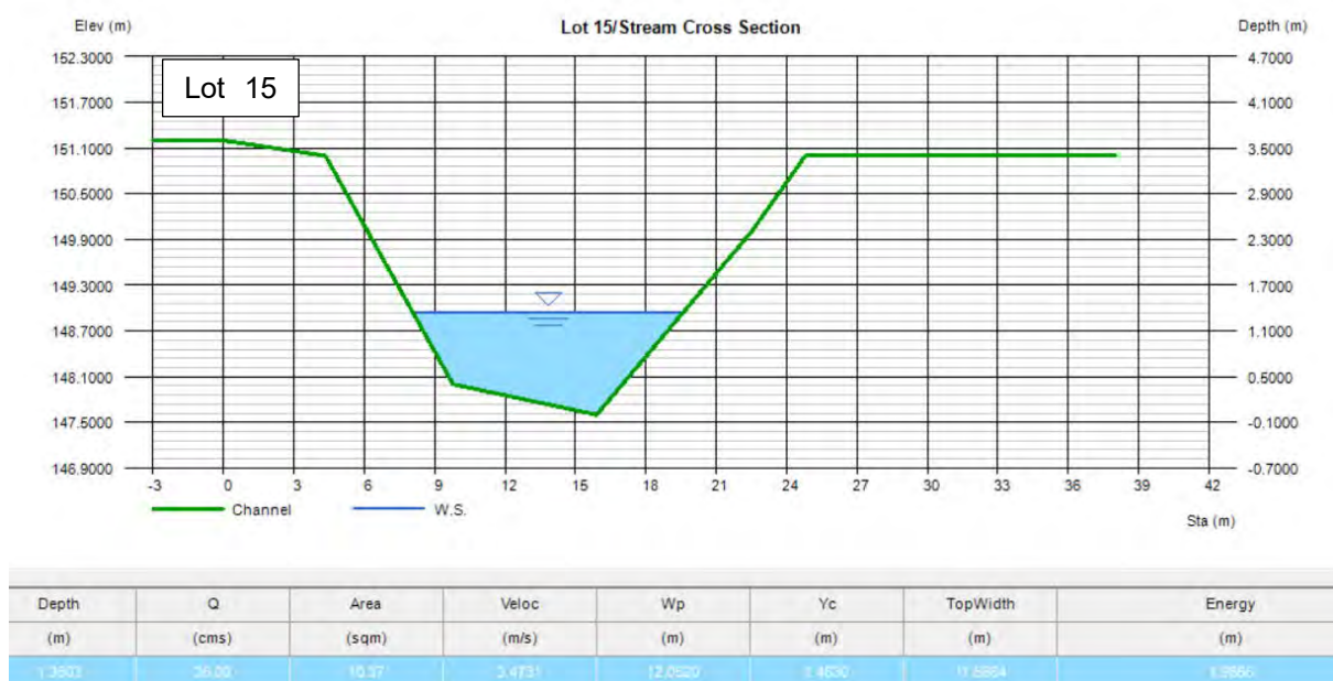
Figure 6. Hydraflow Express Stream model adjacent to Lot 15 existing ground levels.
