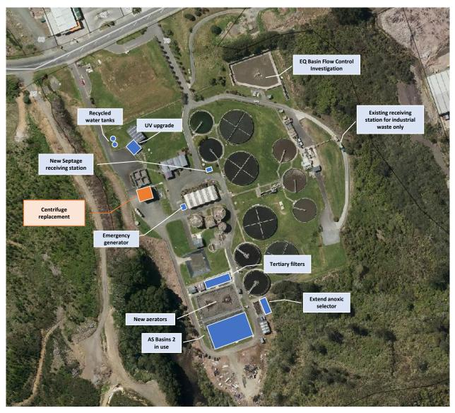
Figure 7 Proposed plant augmentation configuration
