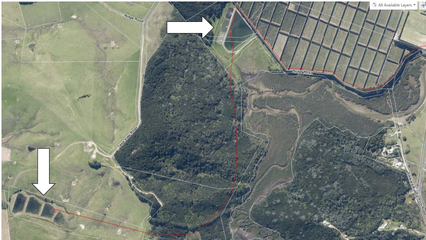
FIGURE 3-2: Aerial photo showing the location of the ponds and constructed wetlands (white arrows). The red line represents the location of the pipes through which wastewater enters and leaves the WWTP.
