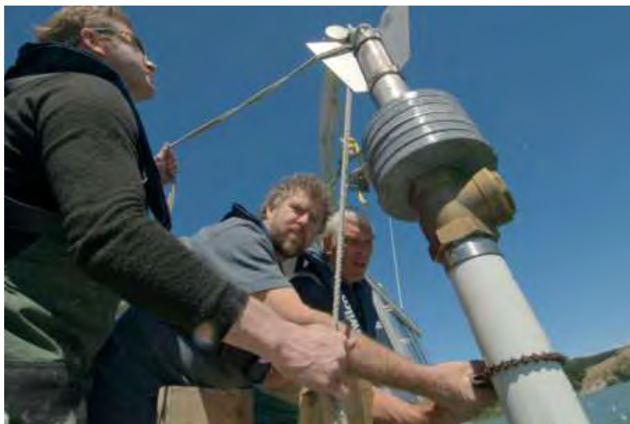
Figure 3-2: Retrieving the Gravity Corer used to collect long cores in the Kaipara Harbour, R.V. Rangitahi III, Kaipara Harbour. March 2010 (photo: Rod Budd, NIWA Hamilton).
